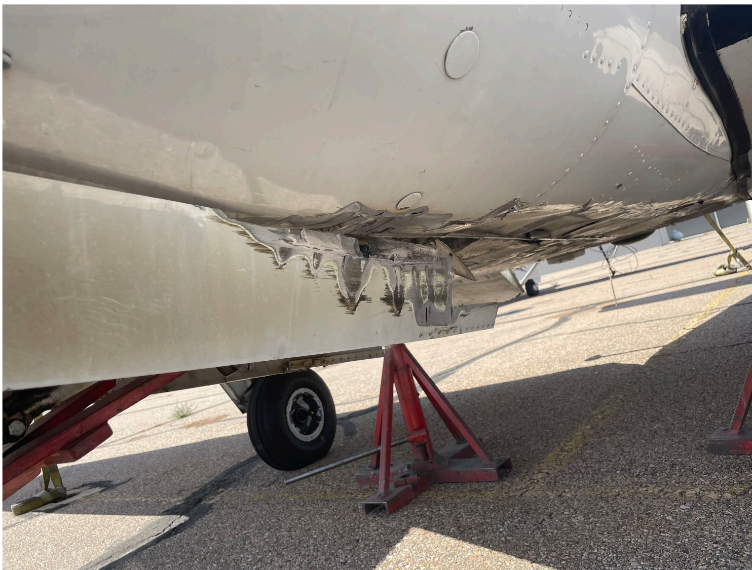
Photograph 3 - Nose Landing Gear Door Damage
