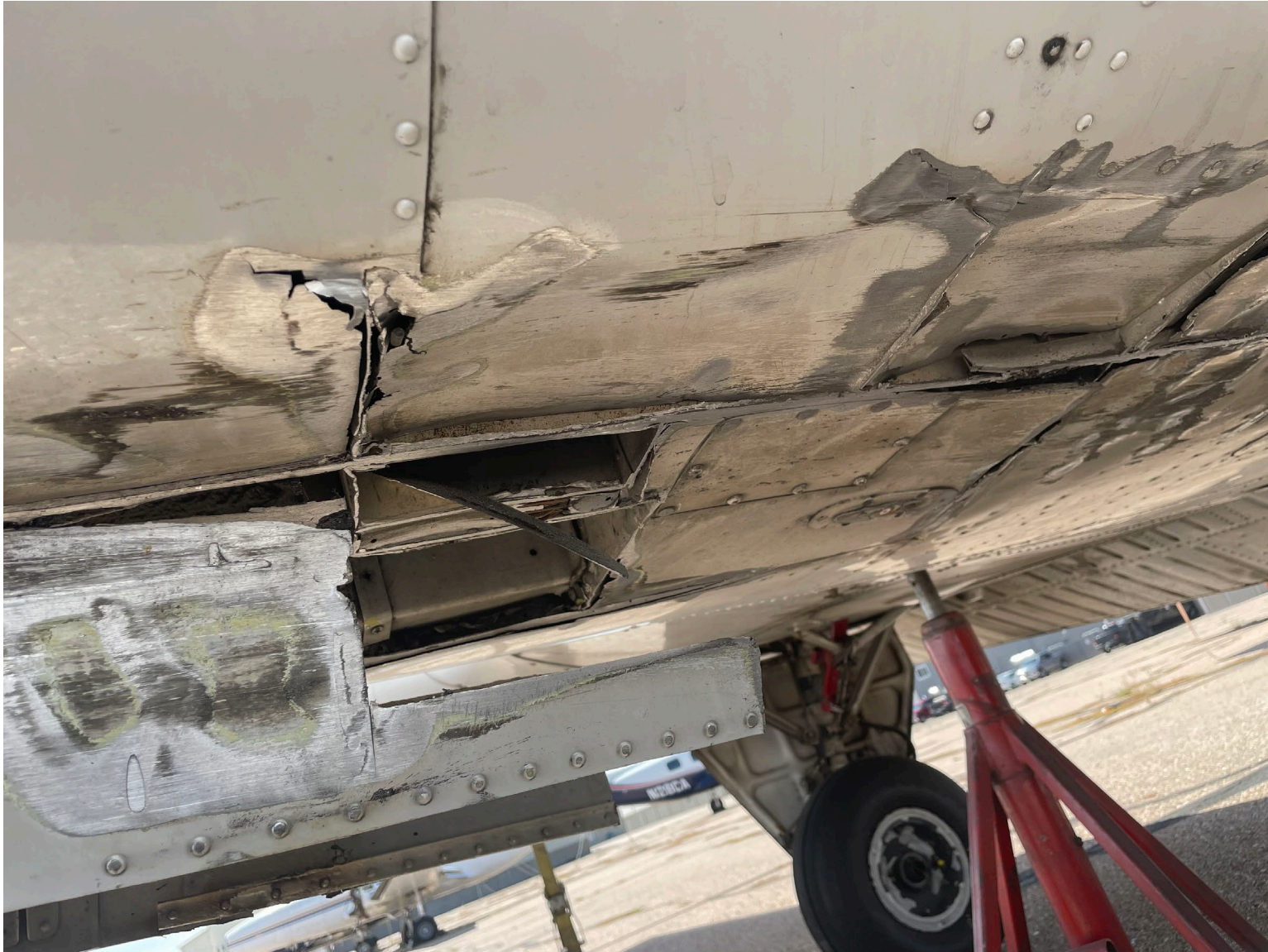
Photograph 2 - Lower Fuselage Damage
