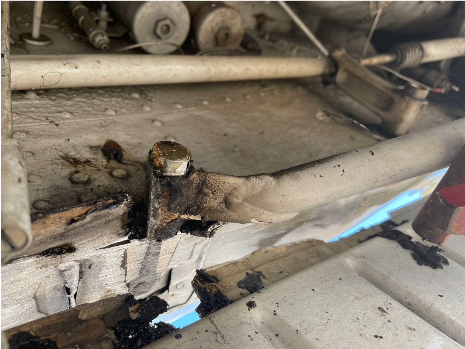
Photograph 4 - Main Landing Gear Actuator
