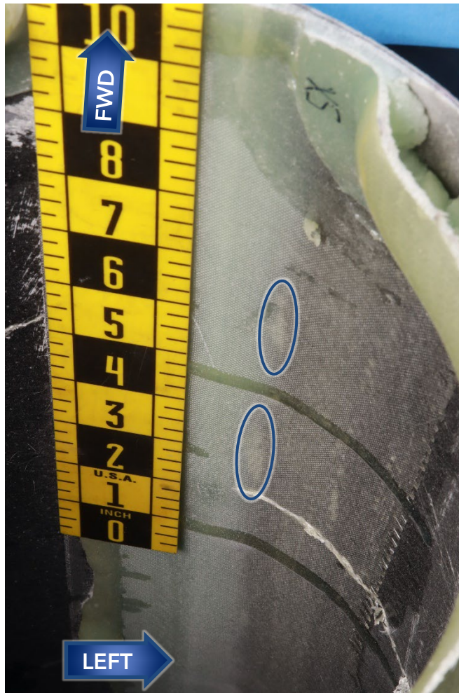
Figure 10. Interior surface of the fuselage at the upper splice location. Areas circled had a lighter appearance consistent with a disbond or void. The longitudinal crack shown in figure 2 was between 7 and 11 inches away from the cut end, which corresponds to the 0 to 4-inch marks on the ruler shown in this image.
