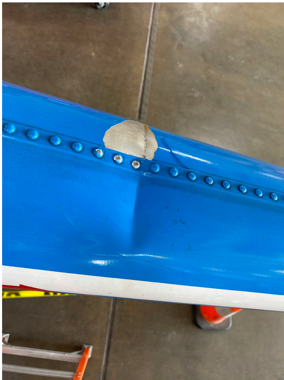
Photo 2 – Tail Boom Damage – (Source: Federal Aviation Administration)
