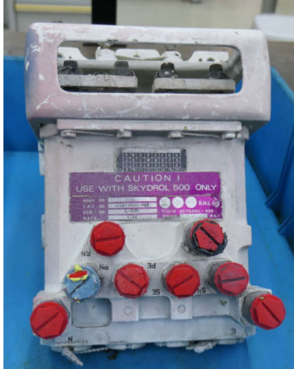
Figure 1 - Brake Power Valve P/N D25W714001-503 S/N IL-019
