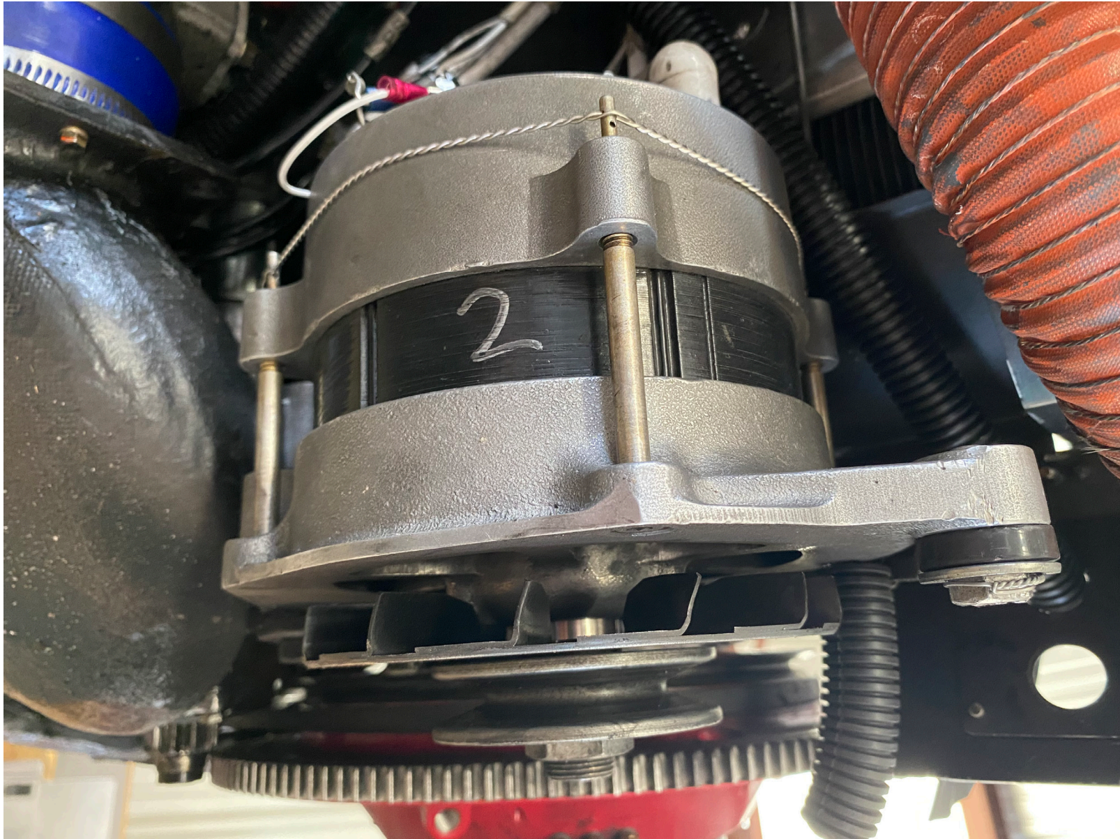
Photograph 4 - Alternator No. 2, belt missing (Courtesy of FAA)
