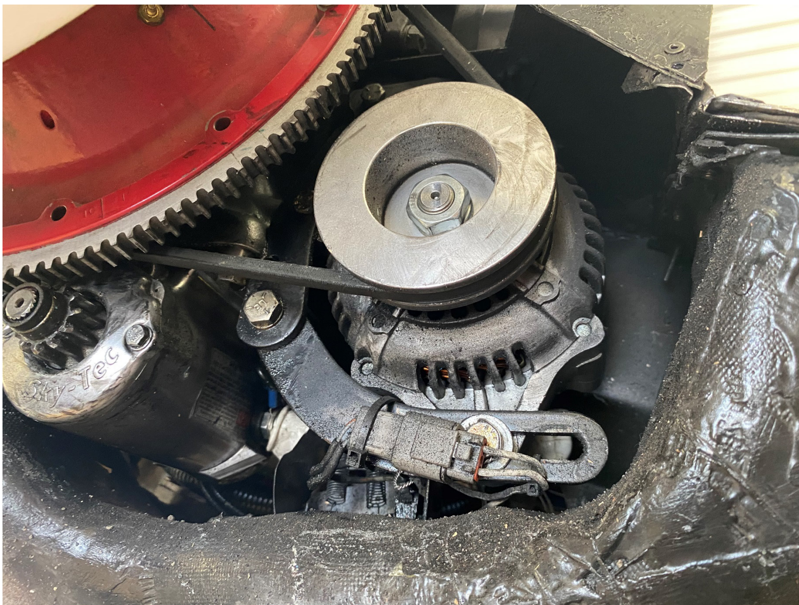
Photograph 6 - Alternator No. 1 (Courtesy of FAA)
