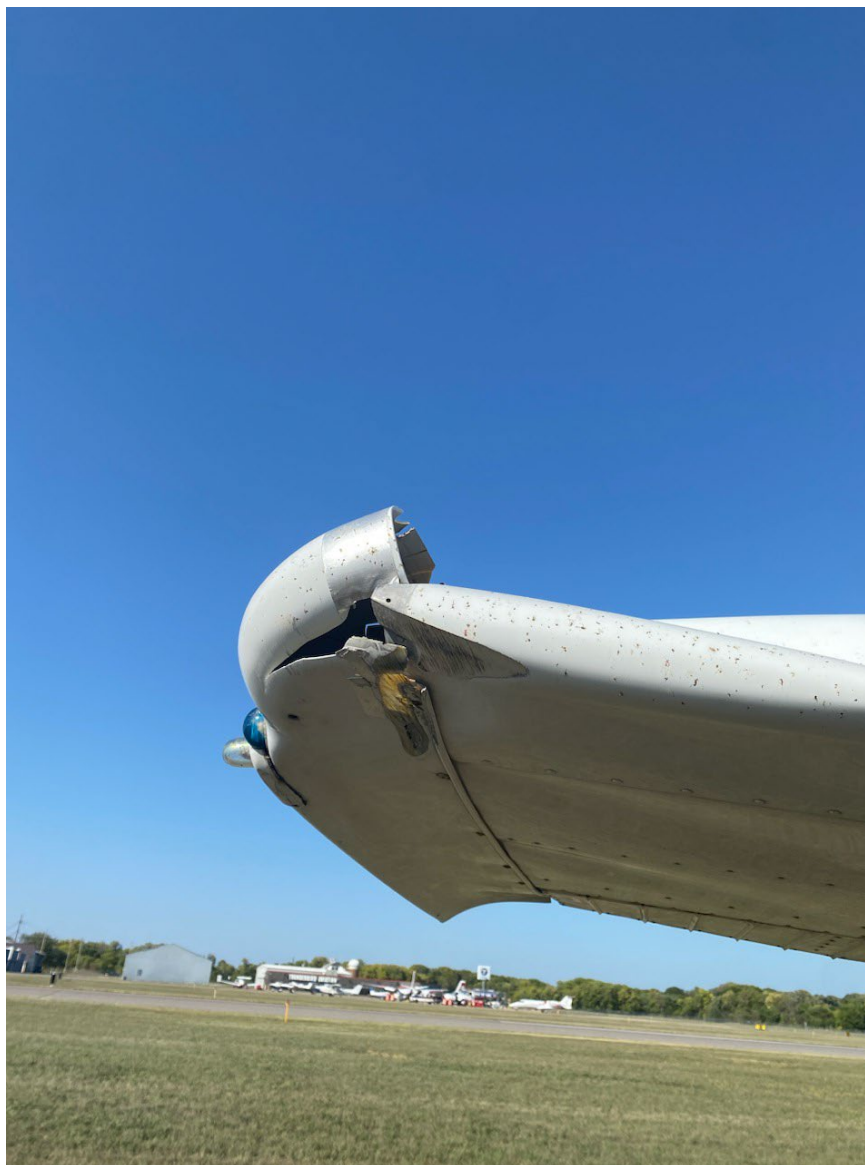
Photograph 1 - Substantially Damaged Right Wing (Courtesy of FAA)
