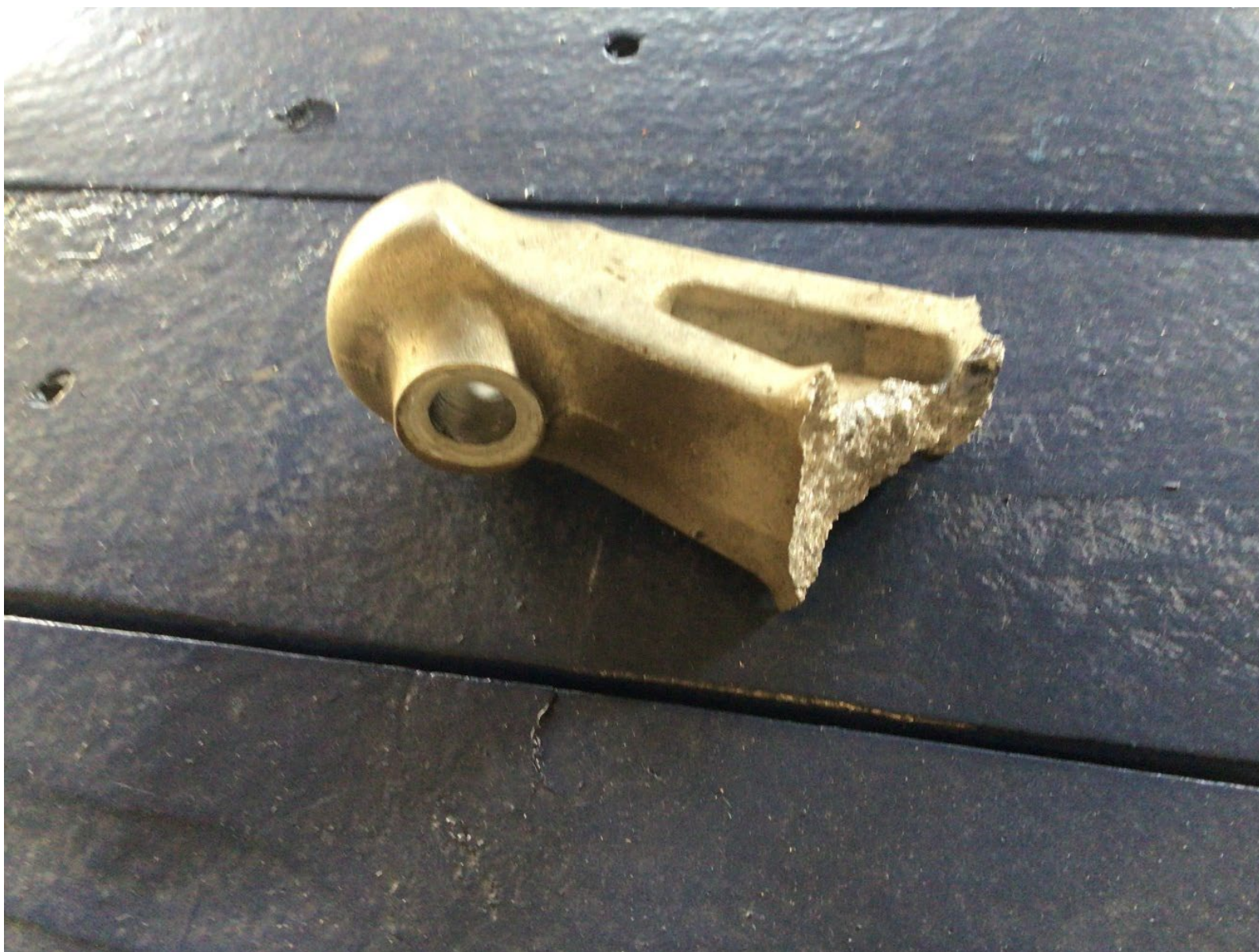
Photograph 8 - View of the fractured engine mount (courtesy of Missouri Aviation, Inc.)
