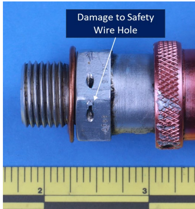
Figure 7. Damage on one of the safety wire holes.
