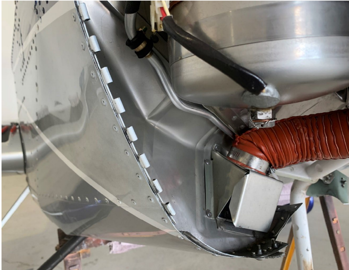
Photograph 2 - View of the firewall (Courtesy of the Federal Aviation Administration)
