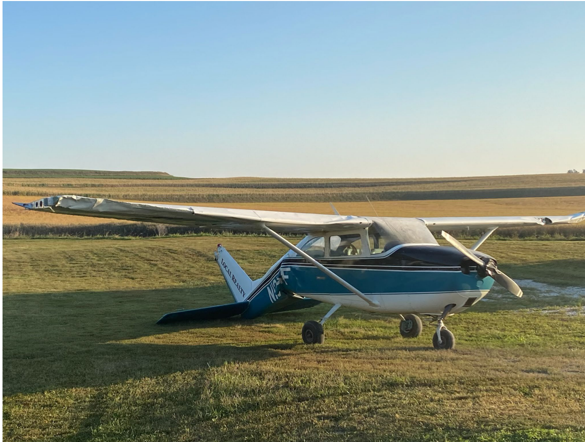
Photograph 2 - Deformation noted to the fuselage and both wings (Courtesy of Pilot)
