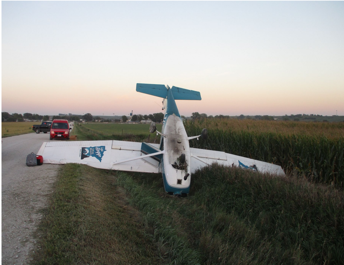
Photograph 1 - Deformation noted to the fuselage and both wings (Courtesy of Sheriff's Office)
