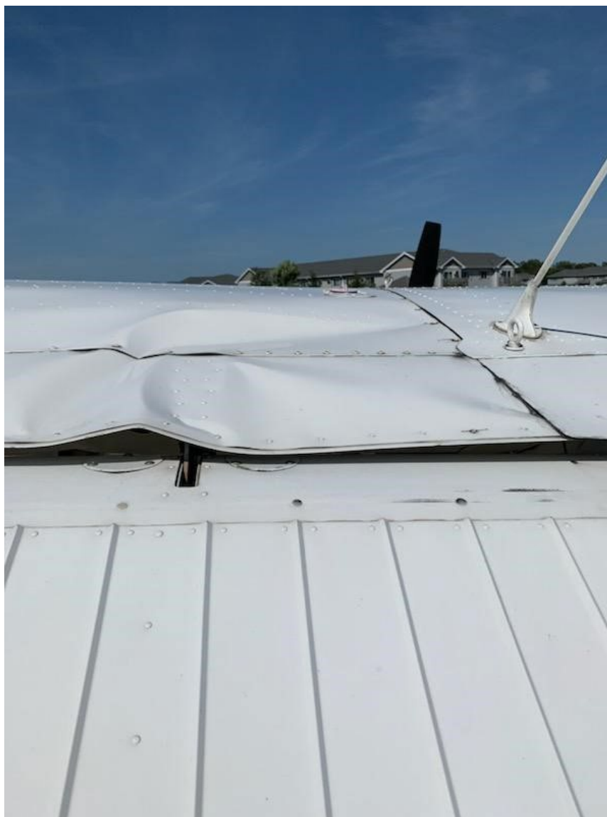
Photograph 1 - Left wing rear spar is bent and buckled (Courtesy of Wisconsin State Patrol)
