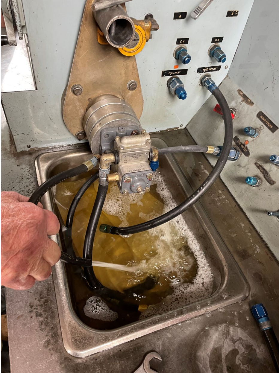
Figure 3. Fuel pump connected to test bench.
