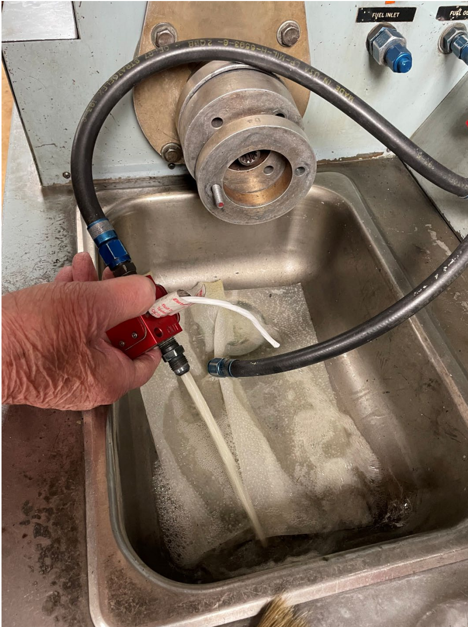
Figure 4. Fuel flow sensor connected to test bench.
