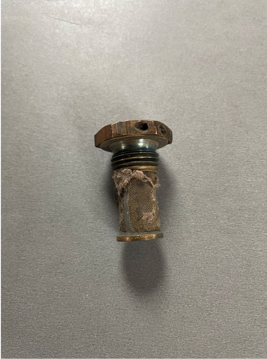
Figure 1 Debris as found on fuel control unit screen.
