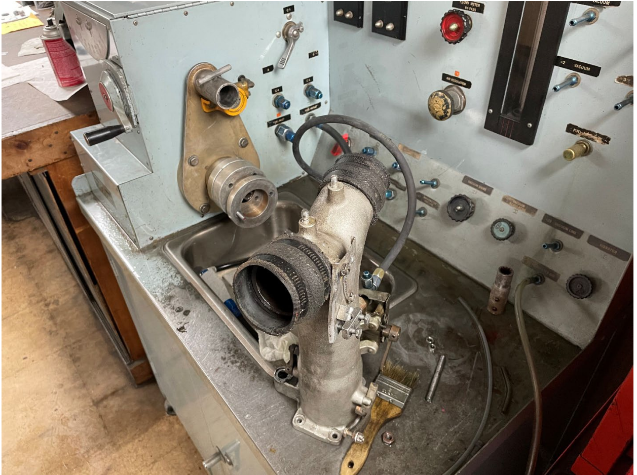
Figure 2. Fuel control unit/throttle body connected to flow bench.
