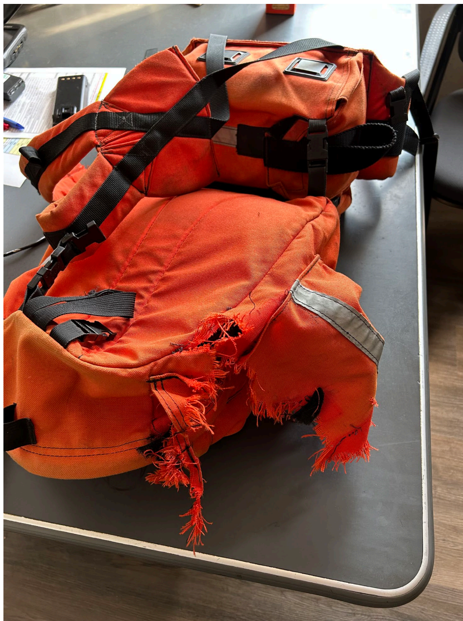
Photo 11 – View of the damaged backpack (courtesy of Brainerd Helicopter Service).
