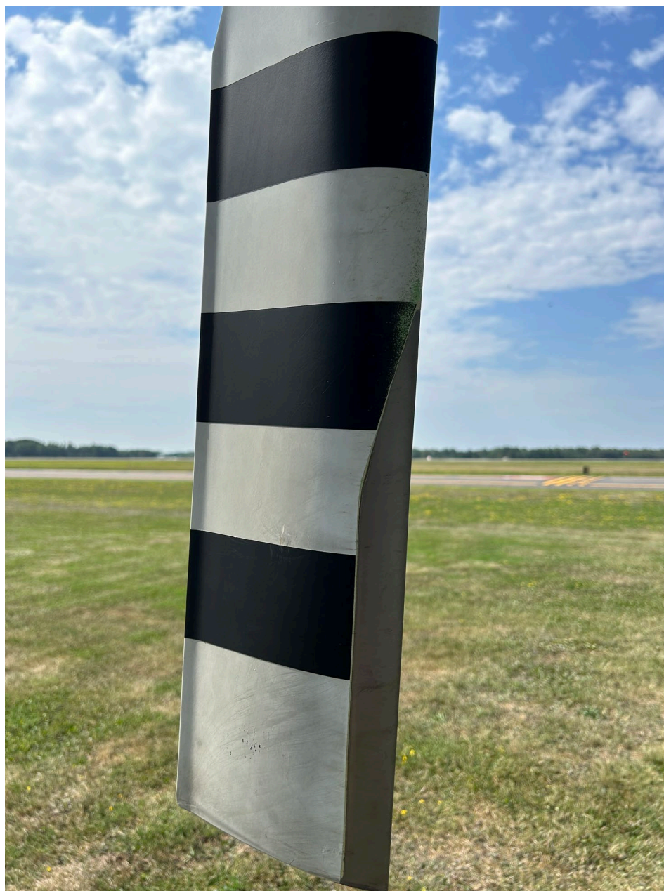
Photo 6 – View of tail rotor blade #1, showing the inward face (courtesy of Brainerd Helicopter Service).
