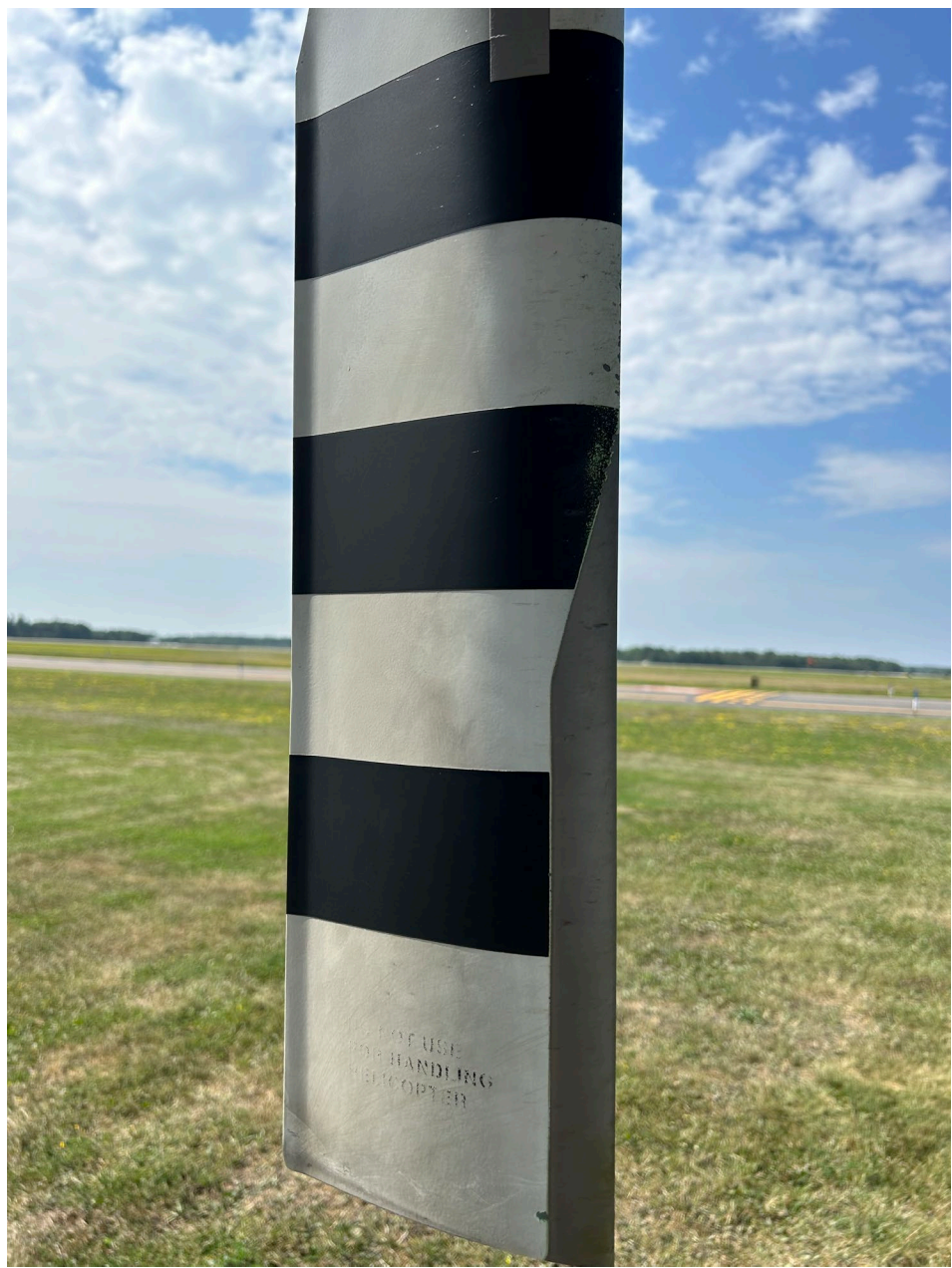
Photo 8 – View of tail rotor blade #2, showing the inward face (courtesy of Brainerd Helicopter Service).
