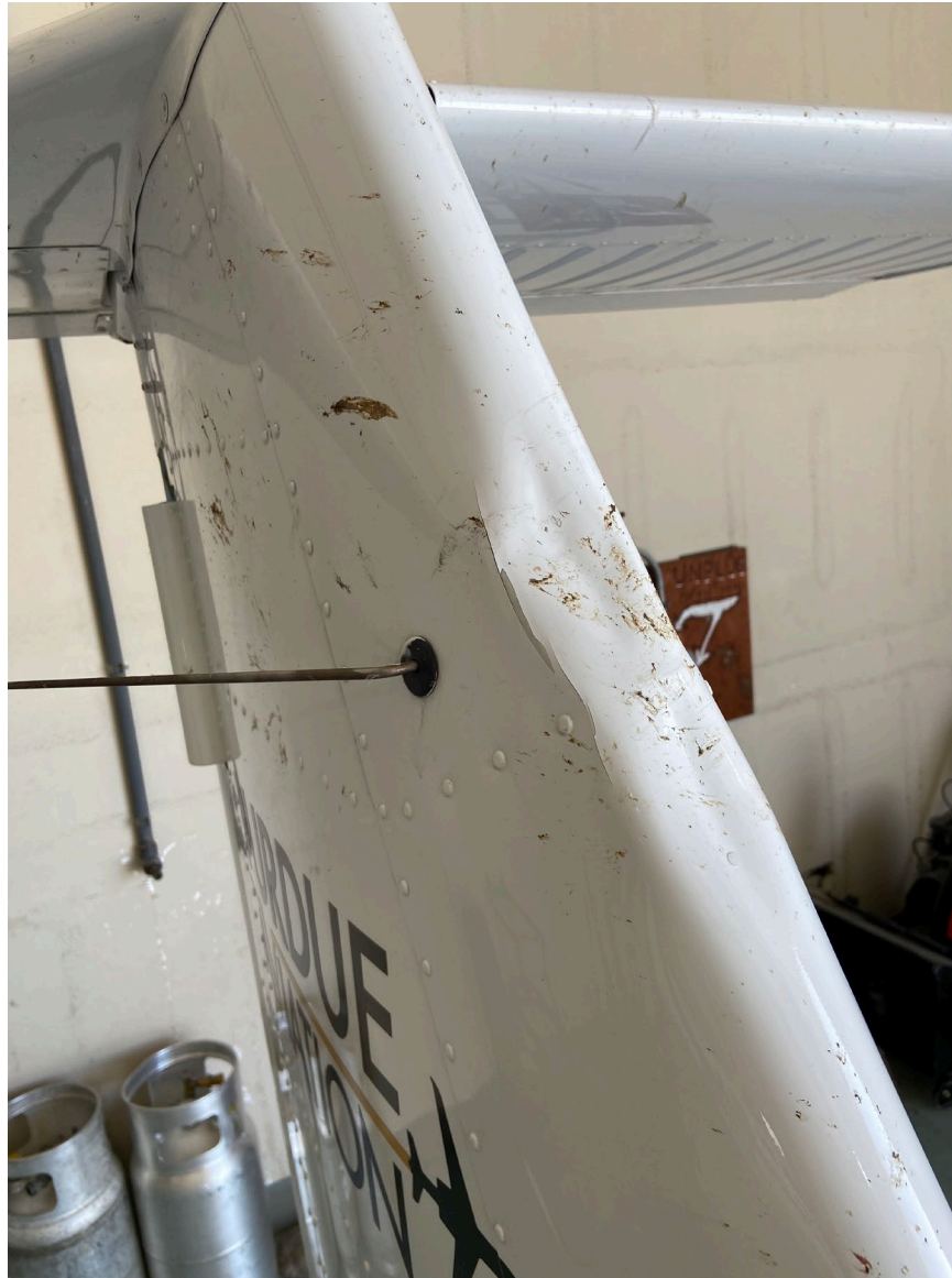
Photograph 1 -Dented Vertical Stabilizer Leading Edge (Courtesy of Purdue Aviation)
