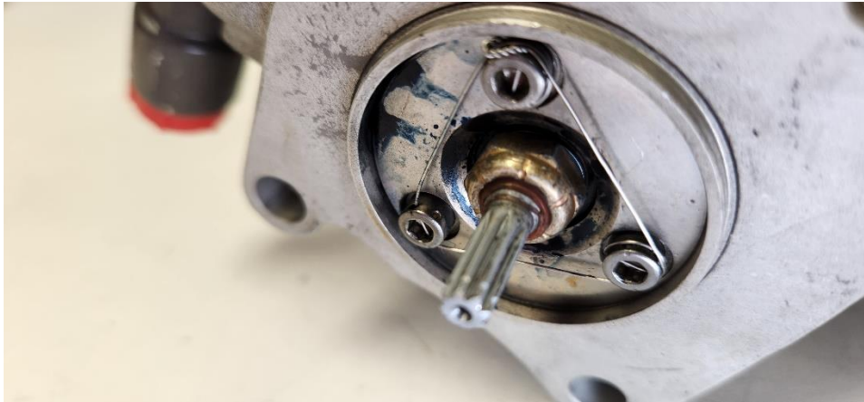
Blue dye found at FCU mating flange between fuel pump and FCU.
