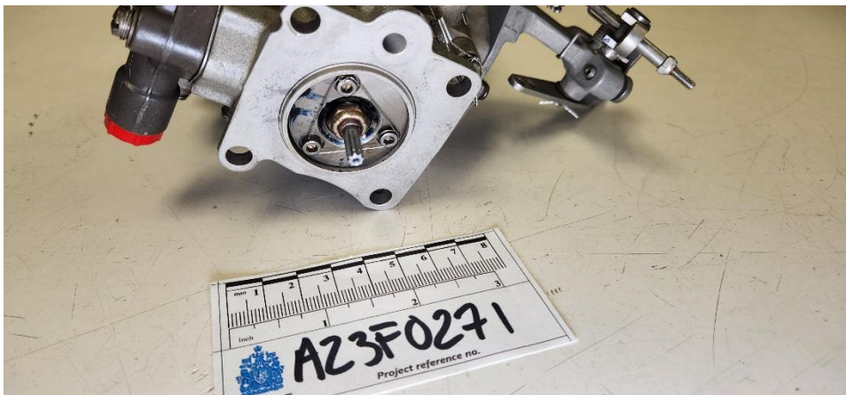
Blue dye found at mating flange between fuel pump and FCU.
