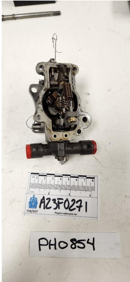
Oil found at mating flange of governing section.
