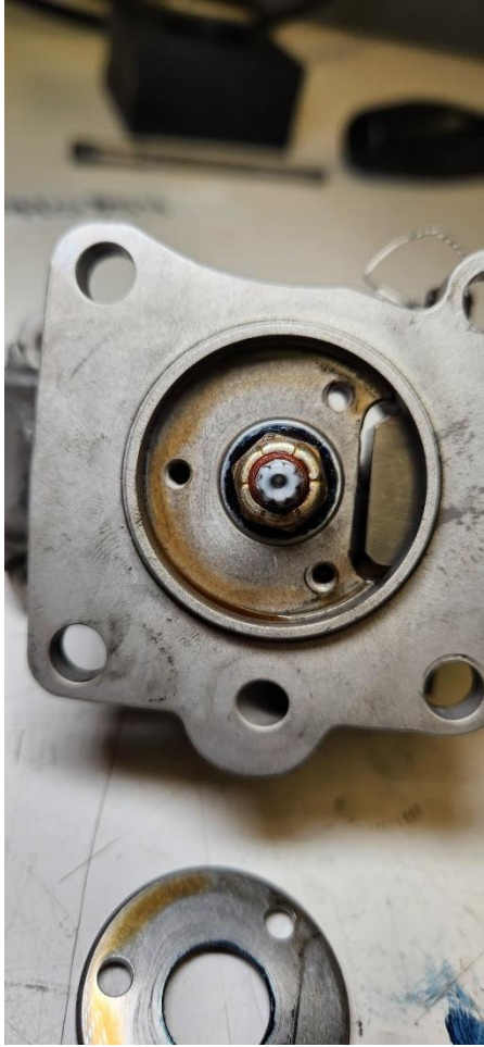
Oil consistent with engine oil found on adapter plate at FCU shaft.
