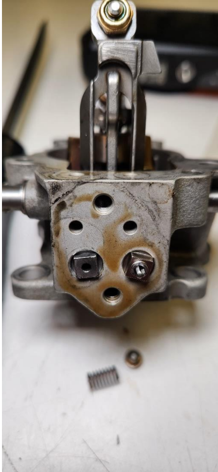
Mating P3/Py flange on governing case found with oil consistent with engine oil.
