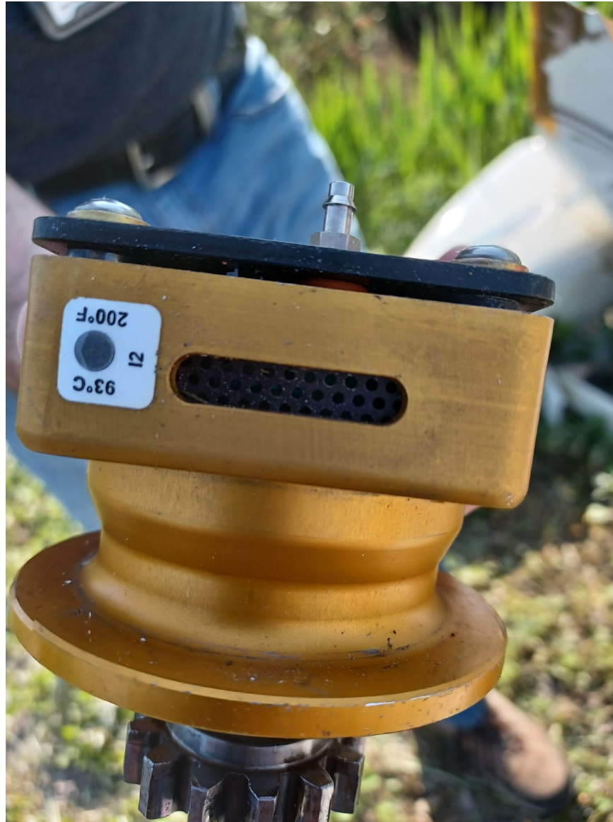
Photograph 2 - Magneto with thermal sticker (Courtesy of Mechanic)
