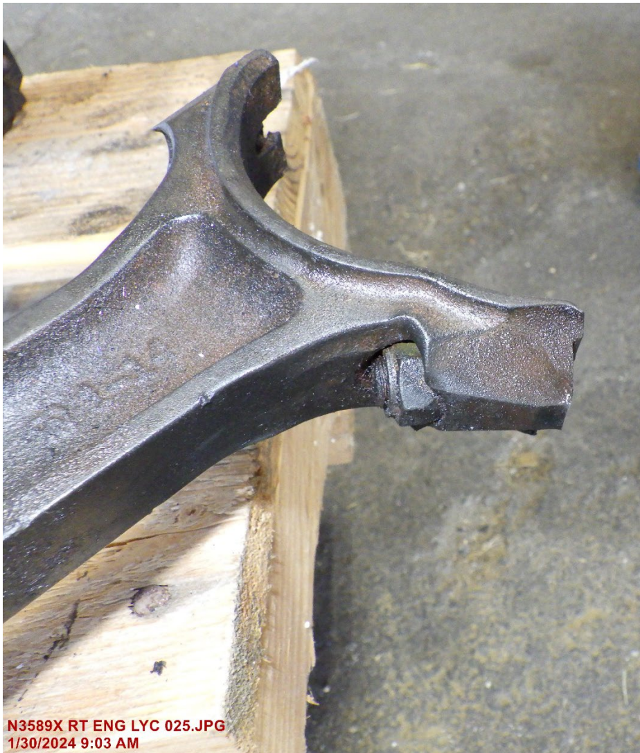
Figure 1 Connecting Rod Arm with Bolt
