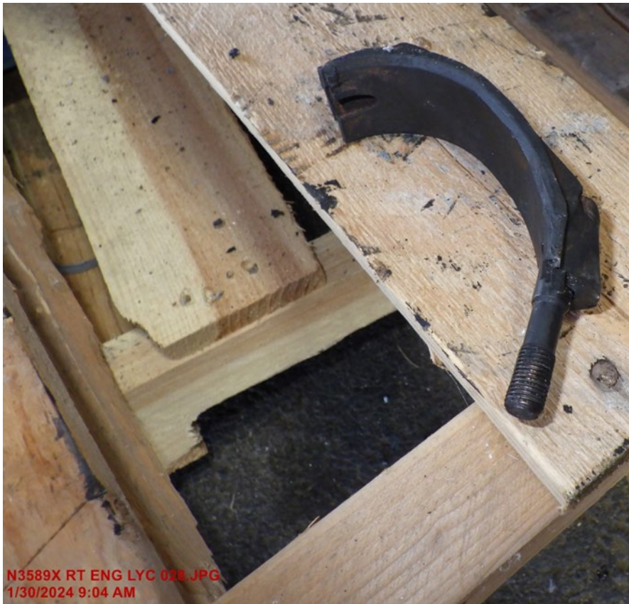
Figure 2 Connecting Rod Cap with Bolt
