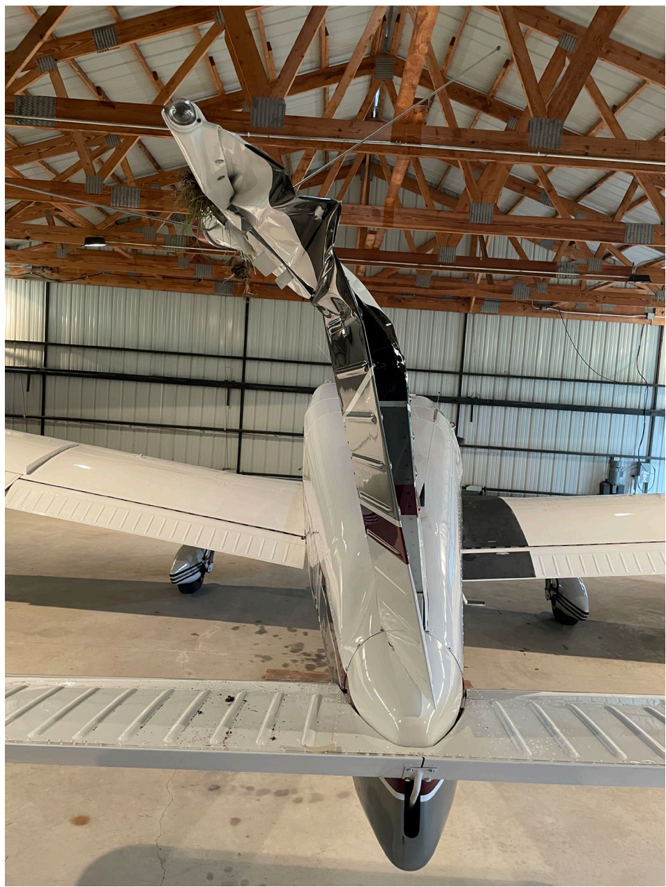
Photo 2 – Vertical stabilizer and rudder damage (Source: FAA)
