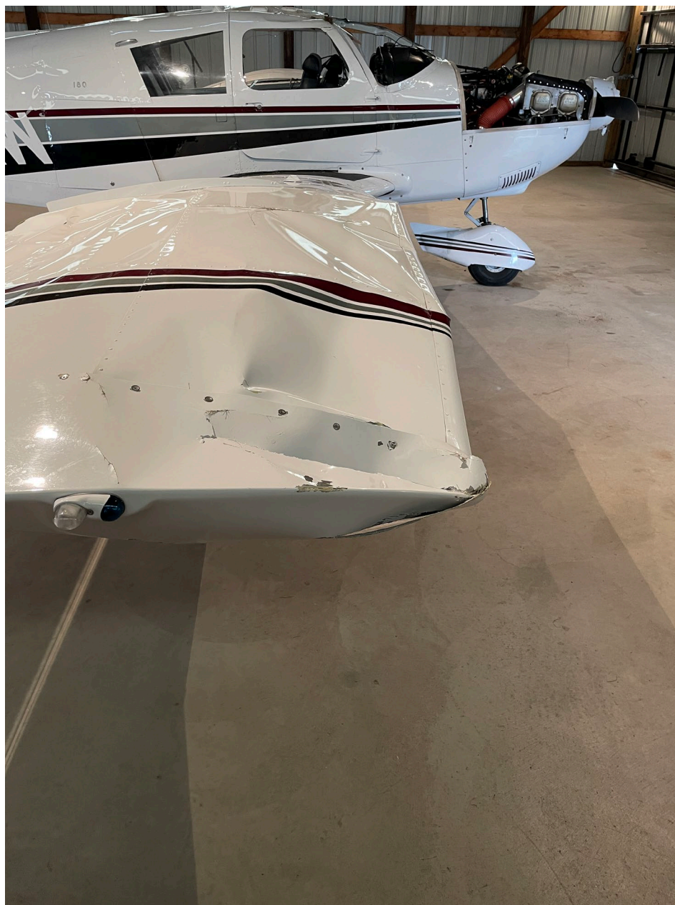
Photo 1 – Right wing damage (Source: FAA)
