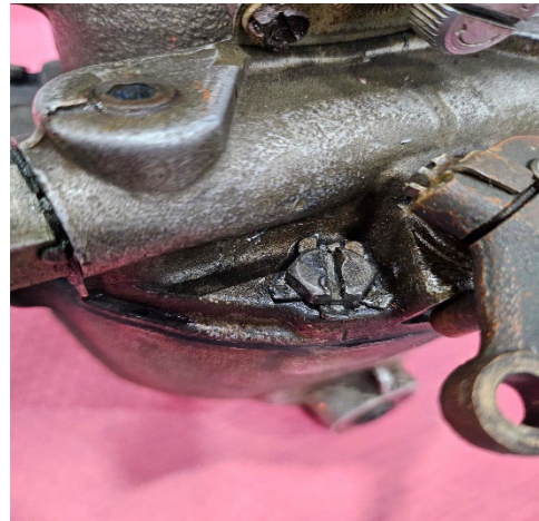
Lock tabs not bent and bolts loose.
