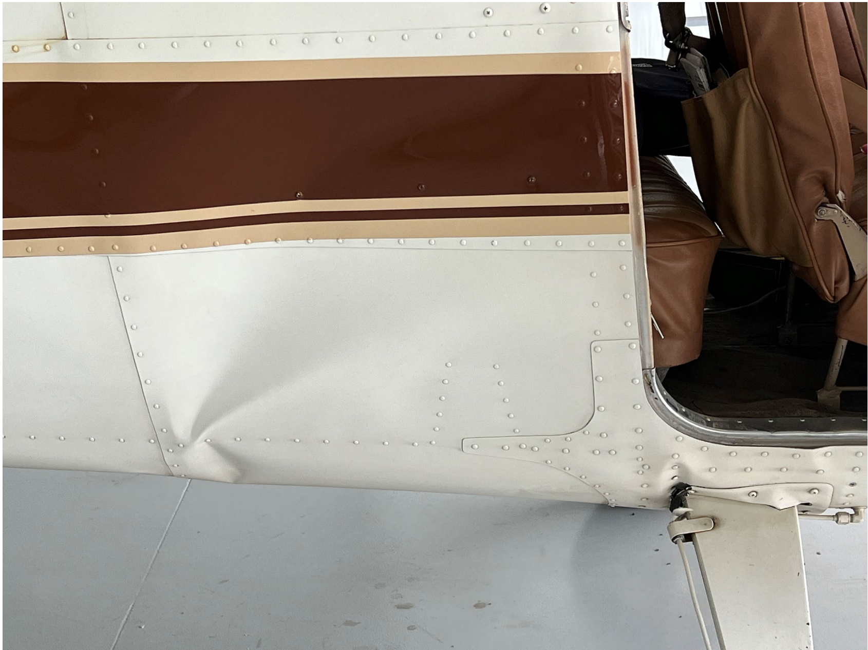
Photo of Fuselage Damage, Courtesy of FAA
