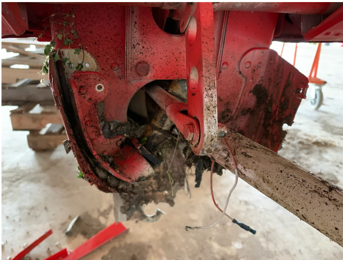
Photograph 2 - Substantial damage to tailwheel supporting structure (Courtesy of FAA)
