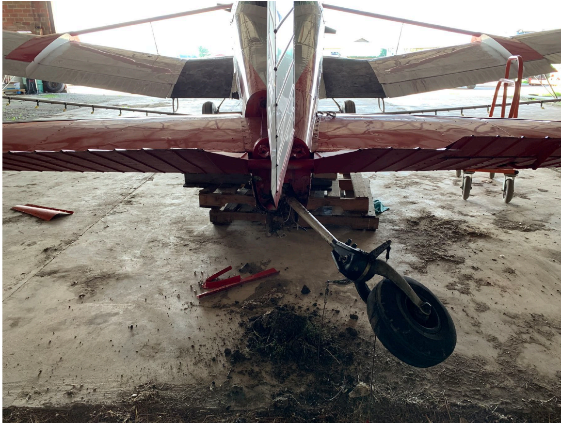
Photograph 1 -Tailwheel assembly displaced to the right (Courtesy of FAA)
