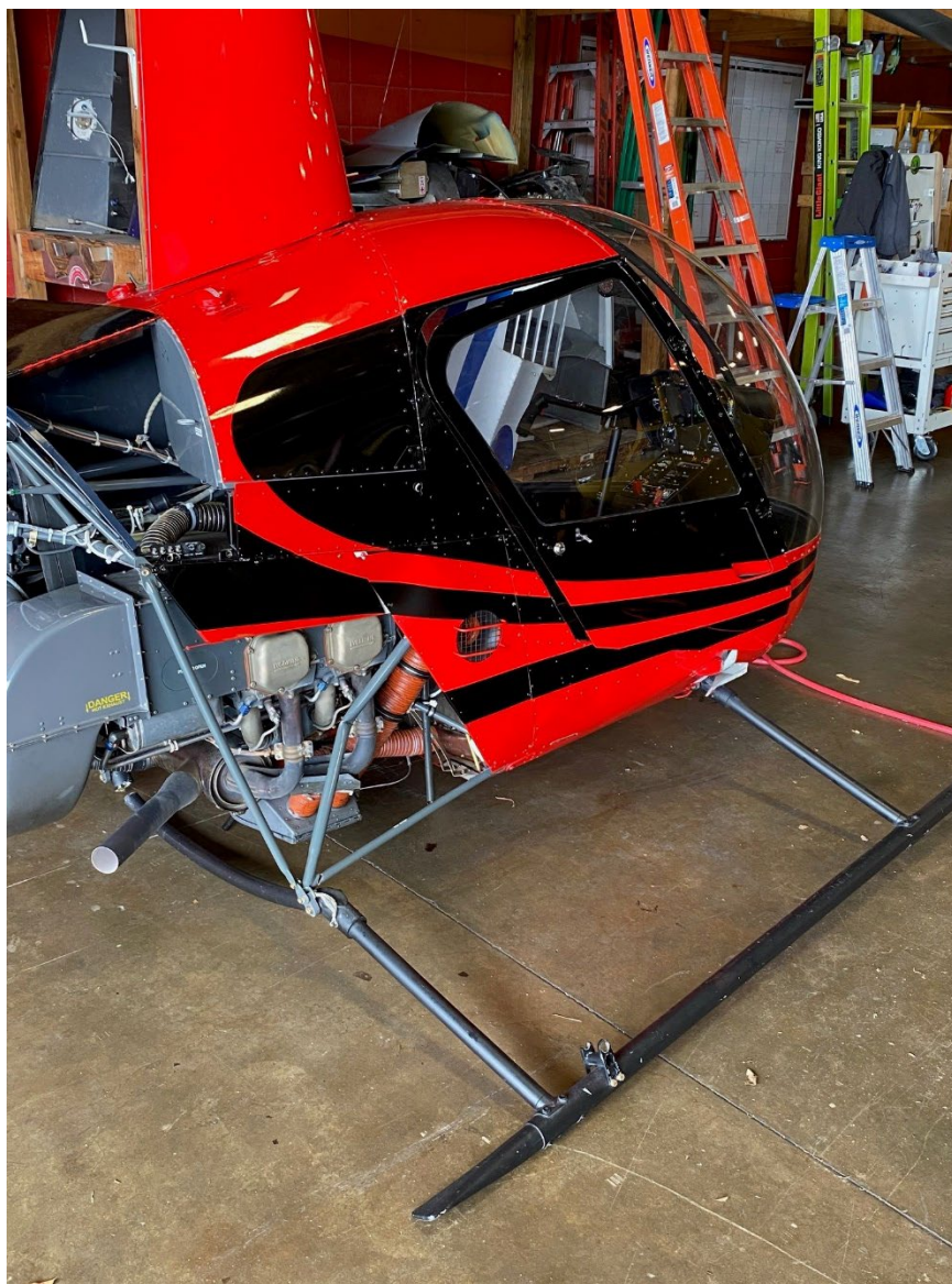
Photograph 3 - deformation to the skids and fuselage tubular structure (Courtesy of FAA)
