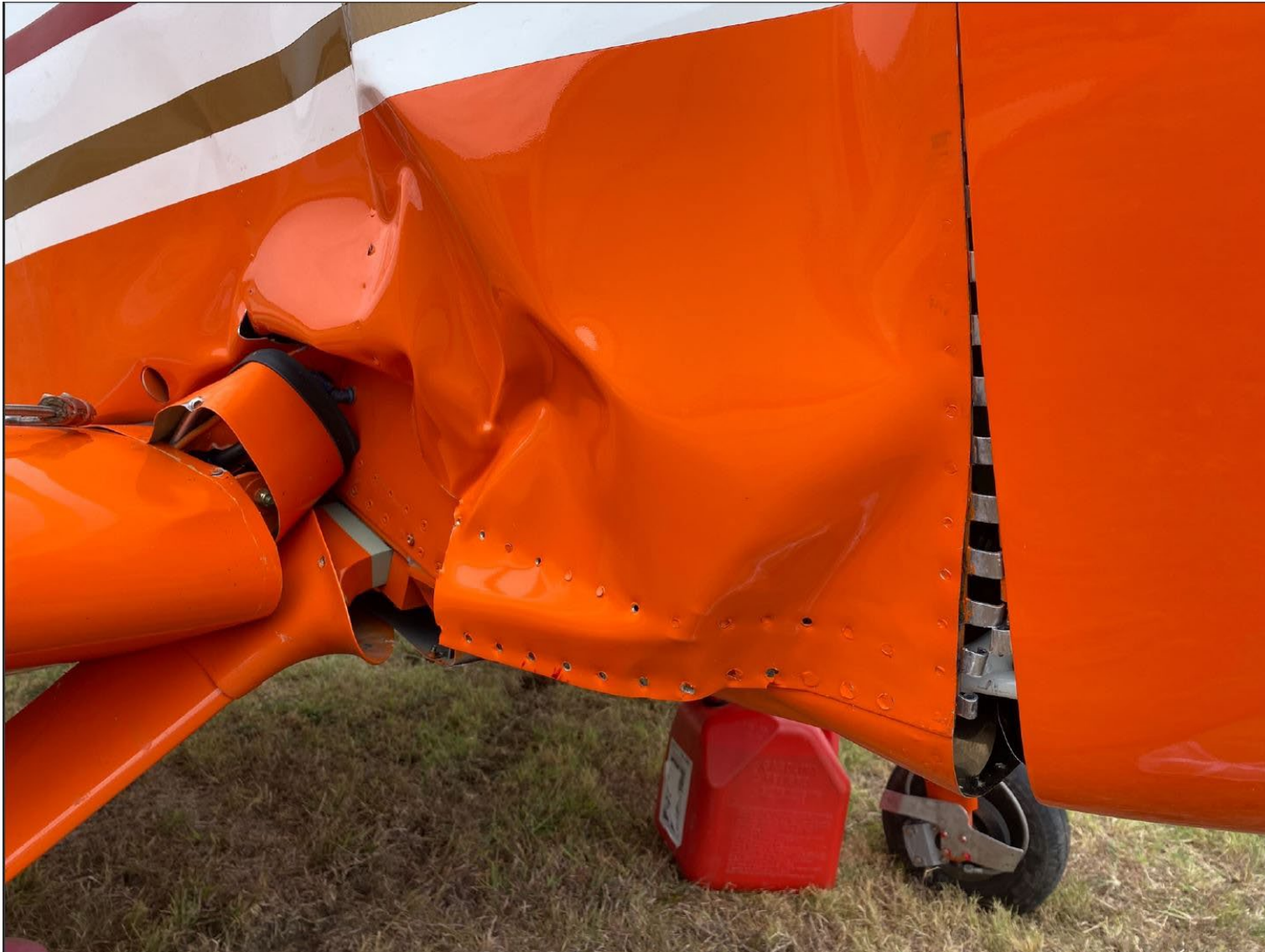
Photograph 1 - R/H View of Damaged Fuselage (Courtesy of FAA)
