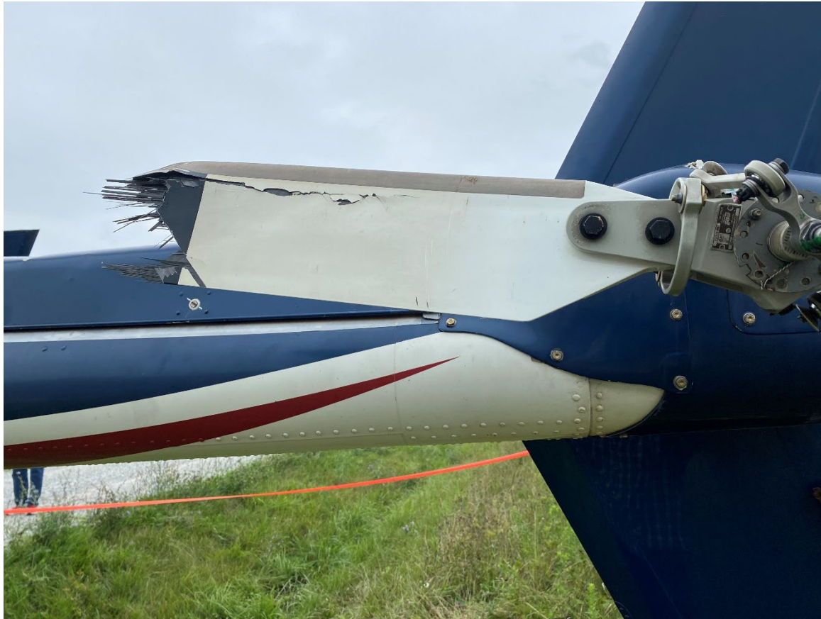
Photograph 10 - View of the damage sustained to the one of the tail rotor blades (Courtesy of the Federal Aviation Administration)
