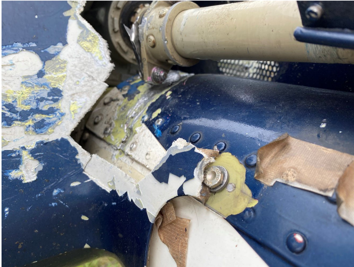
Photograph 8 - View of the damage sustained to the tail boom and the tail rotor driveshaft. (Courtesy of the Federal Aviation Administration)
