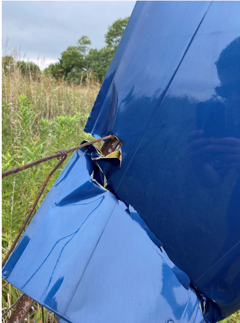
Photograph 7 - View of the vertical stabilizer and the fence at the accident site, during day conditions (Courtesy of the Federal Aviation Administration)
