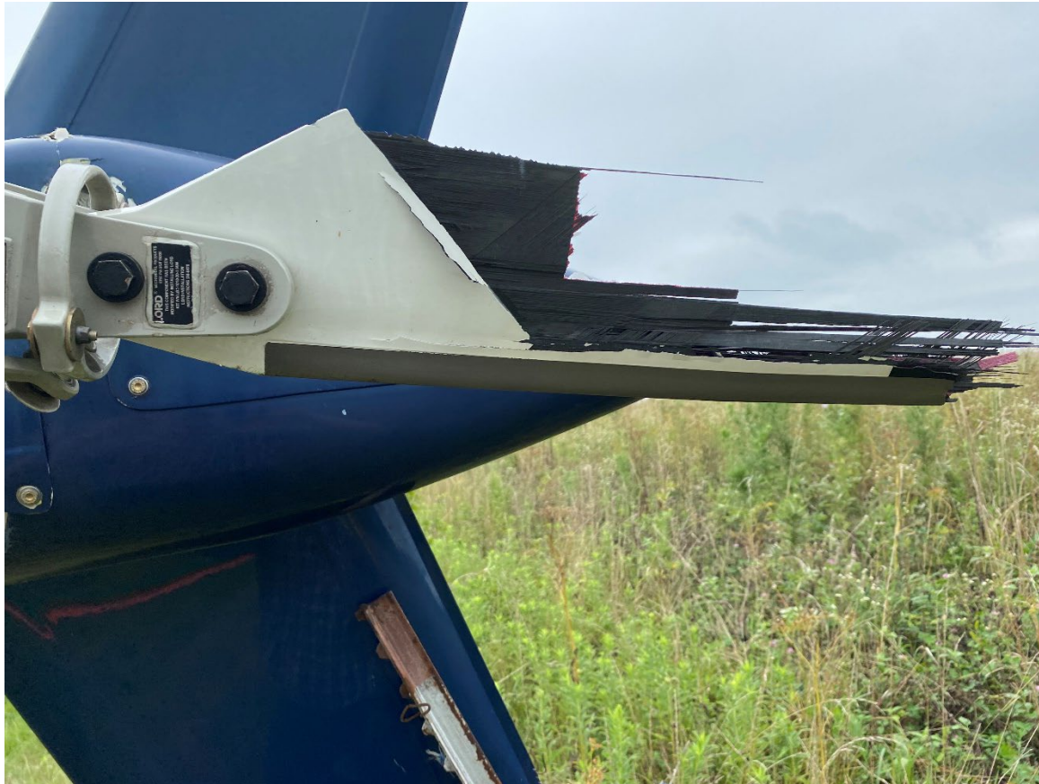
Photograph 9 - View of the damage sustained to one of the tail rotor blades (Courtesy of the Federal Aviation Administration)
