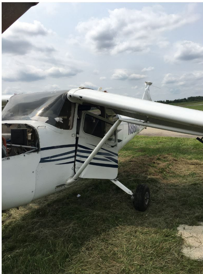
Photograph 2 - Damaged Left Wing and Lift Strut (Courtesy of FAA)
