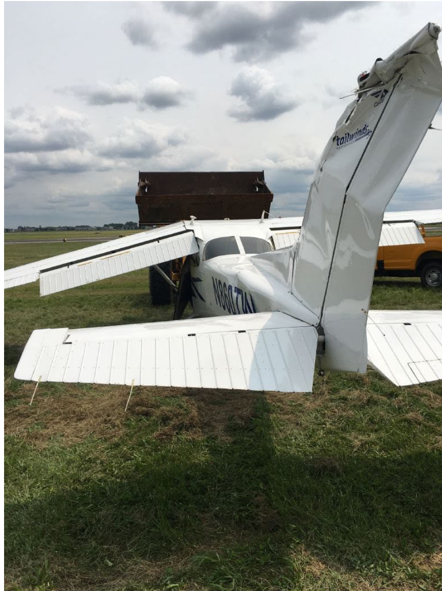
Photograph 1 -Damaged Empennage (Courtesy of FAA)
