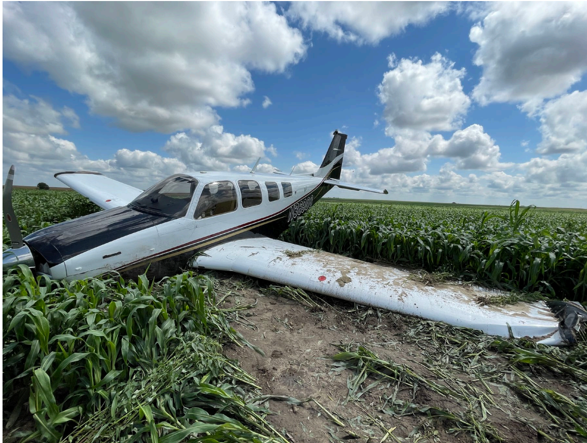
Photograph 1 - Airplane with substantial damage to left wing (Courtesy of Federal Aviation Administration (FAA))
