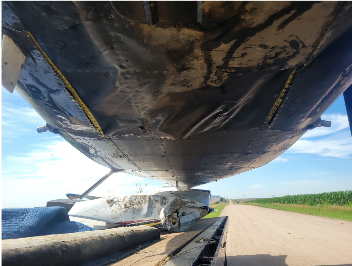
Photograph 2 - Underside of airplane with substantial damage to the fuselage (Courtesy of FAA)
