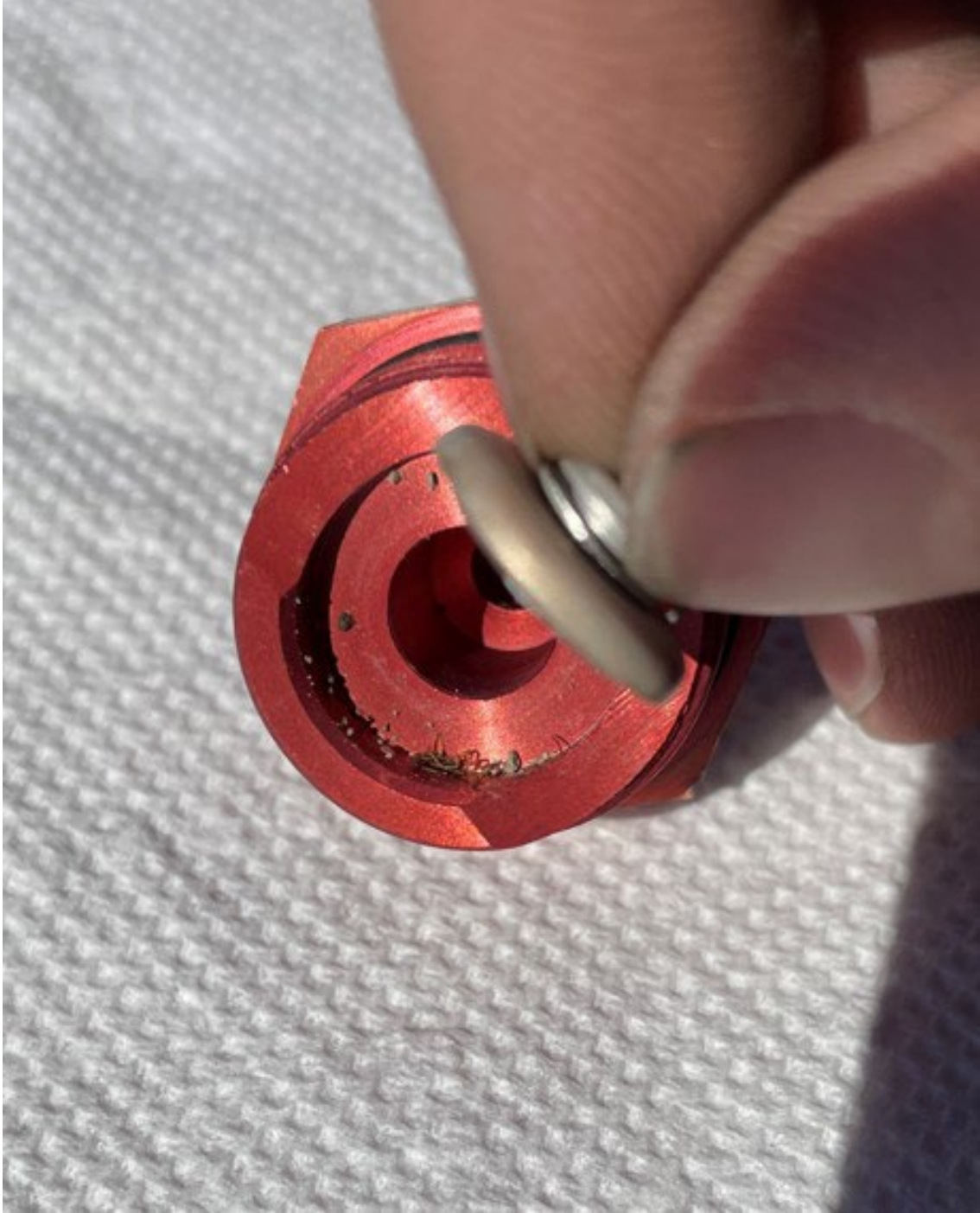
Figure 4: Left wing fuel vent check valve
