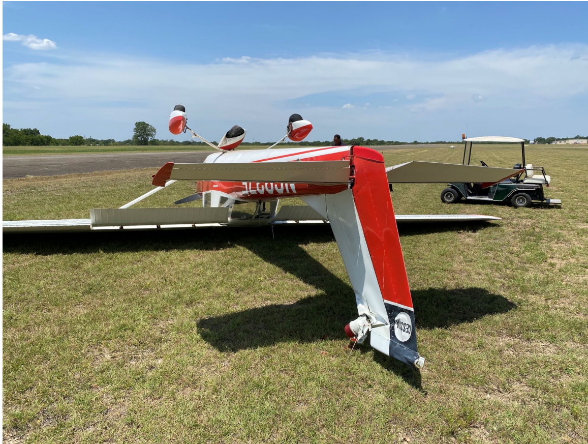
Photograph 2 - Deformation noted to the rudder and vertical stabilizer (Courtesy of FAA)
