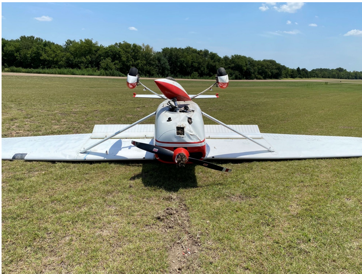
Photograph 1 - Front view of airplane and deformation noted to the left wing (Courtesy of FAA)
