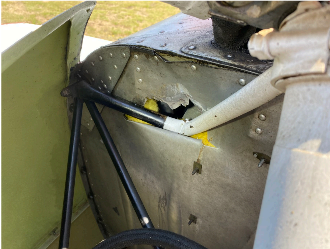
Photograph 3 - Tears in the firewall and deformation to the engine mount (Courtesy of FAA)
