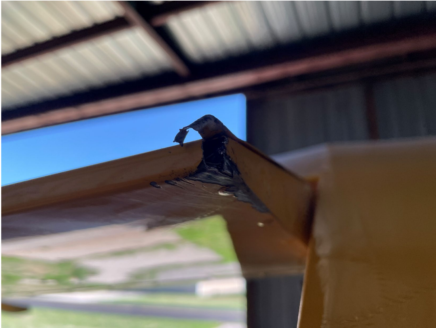
Photograph 2 - Right aileron, outboard trailing-edge damage (Courtesy of FAA)
