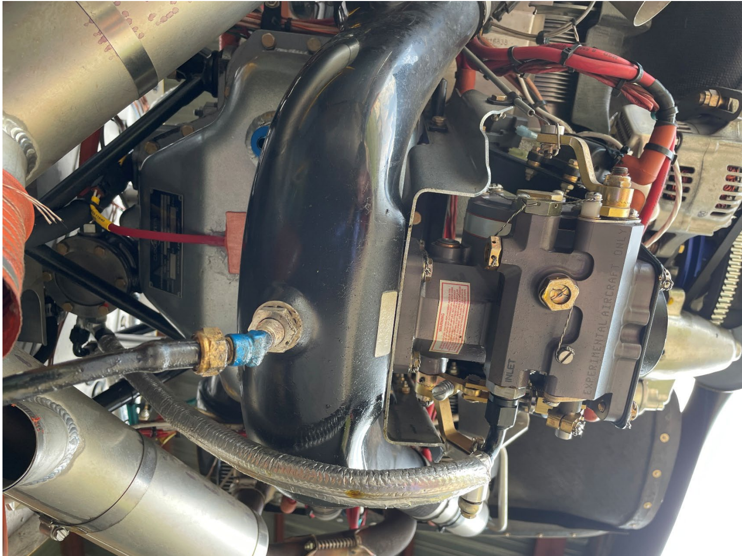
Photograph 5 - Induction airbox and fuel servo detail; throttle and mixture linkages and fuel supply line visible (Courtesy of FAA)
