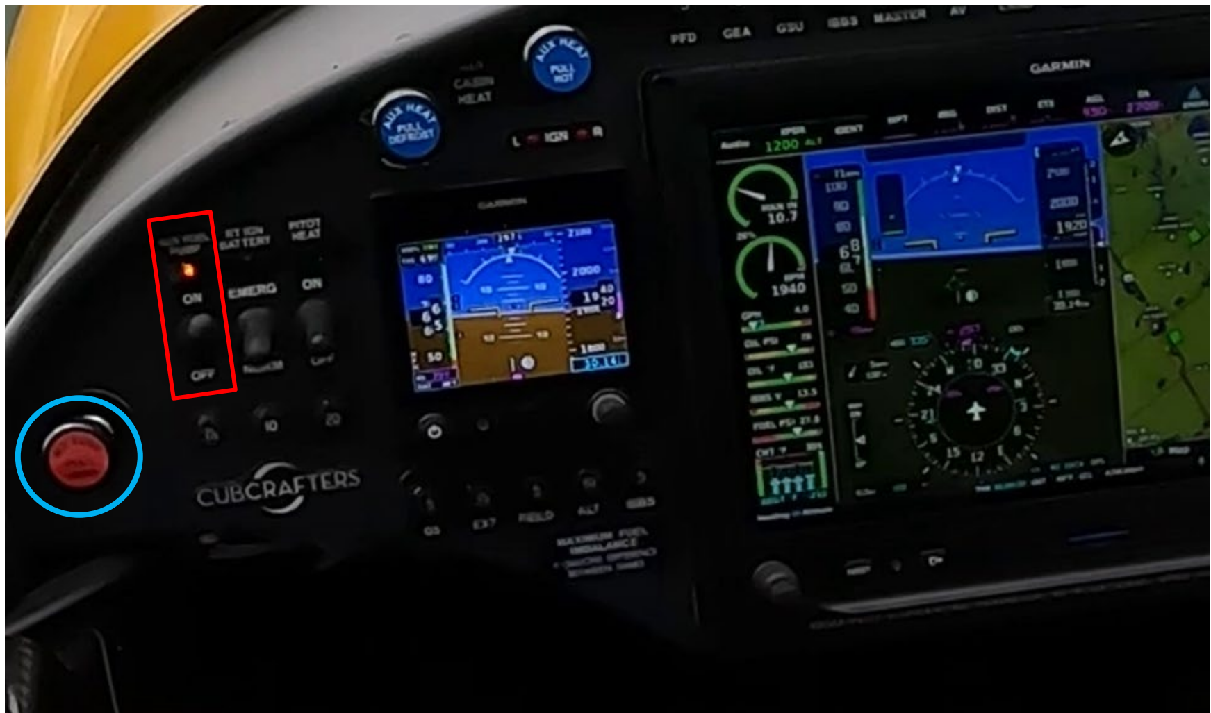
Figure 2. Aux fuel pump (red rectangle) and mixture control knob (blue circle). Screenshot taken at 16:54:17 CDT.
