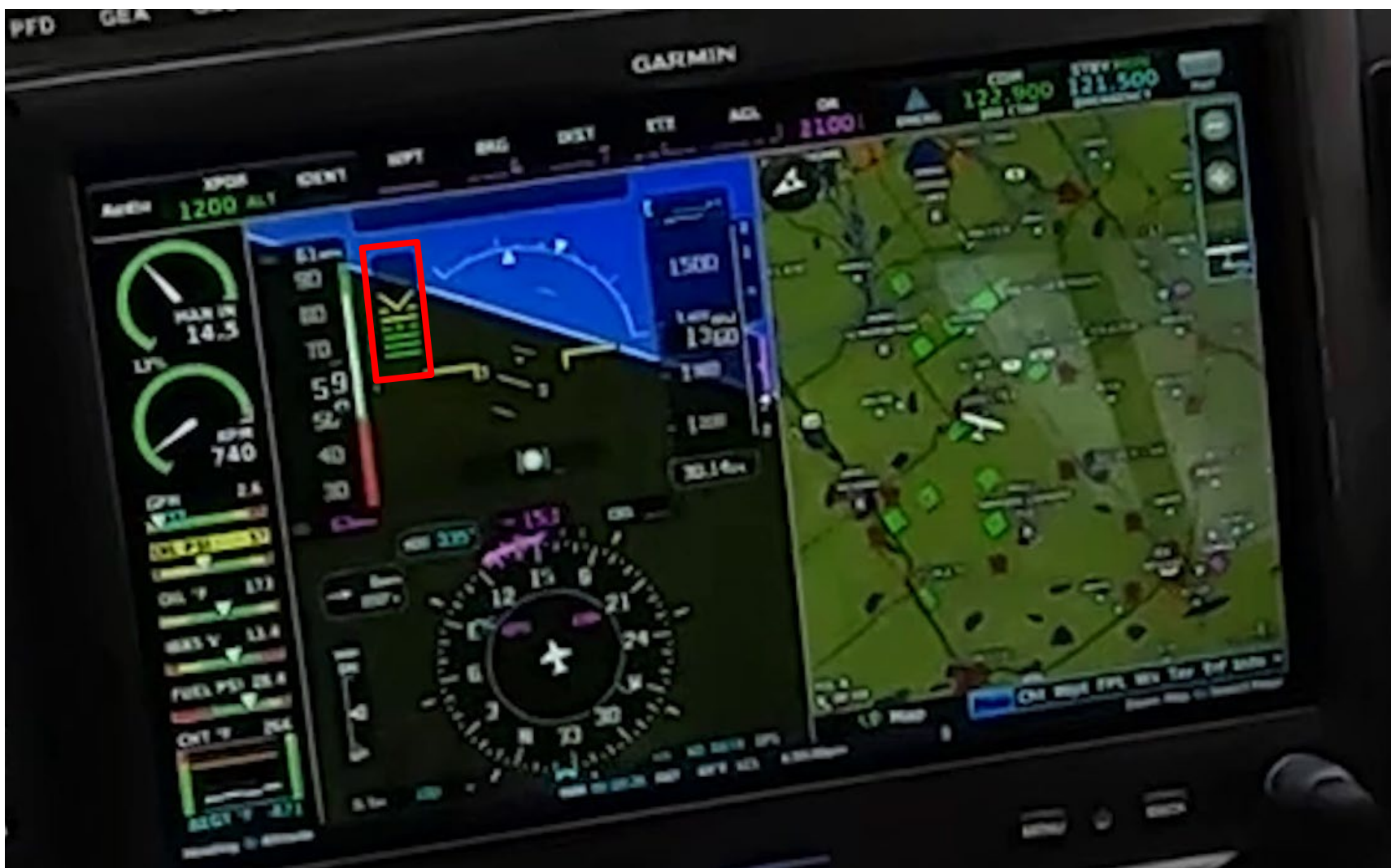
Figure 4. Garmin G3X AOA visual alert for pilots (red rectangle). Screenshot taken at 16:55:06 CDT.
