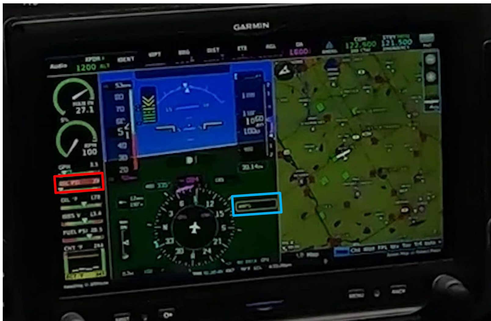
Figure 8. Garmin G3X PFD display with oil pressure red warning (red rectangle) and CAS AMPS yellow caution (blue rectangle). Screenshot taken at 16:55:29 CDT.
