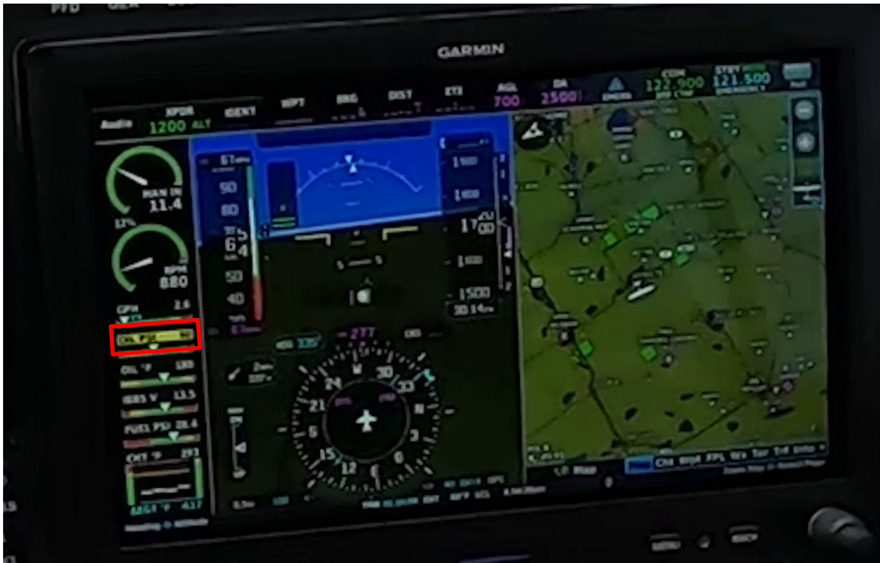
Figure 3. Garmin G3X PFD display with oil pressure yellow caution (red rectangle). Screenshot taken at 16:54:40 CDT.
