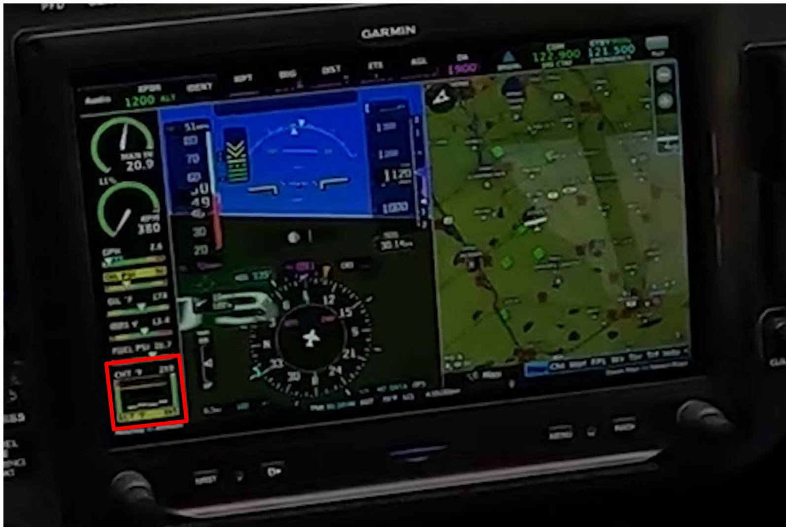
Figure 7. Garmin G3X PFD display with EGT yellow caution (red rectangle). Screenshot taken at 16:55:23 CDT.
