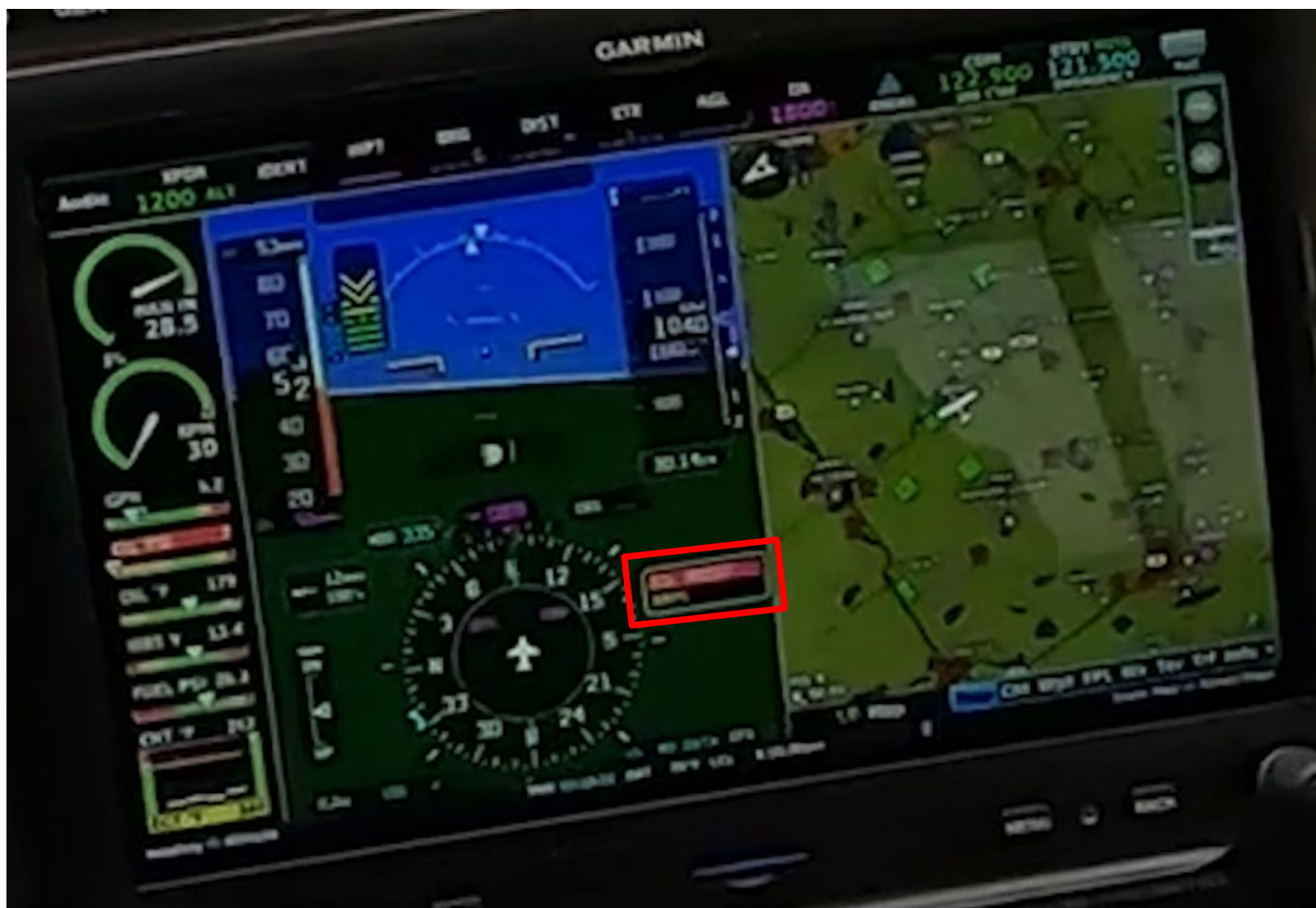
Figure 9. Garmin G3X PFD display with CAS OIL PRESS red warning (red rectangle). Screenshot taken at 16:55:31 CDT.
