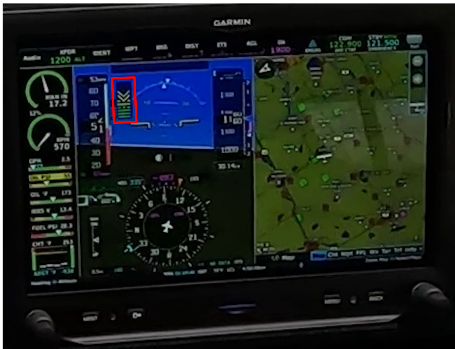
Figure 6. AOA visual alert on Garmin G3X with two chevrons (red rectangle). Screenshot taken at 16:55:20 CDT.
