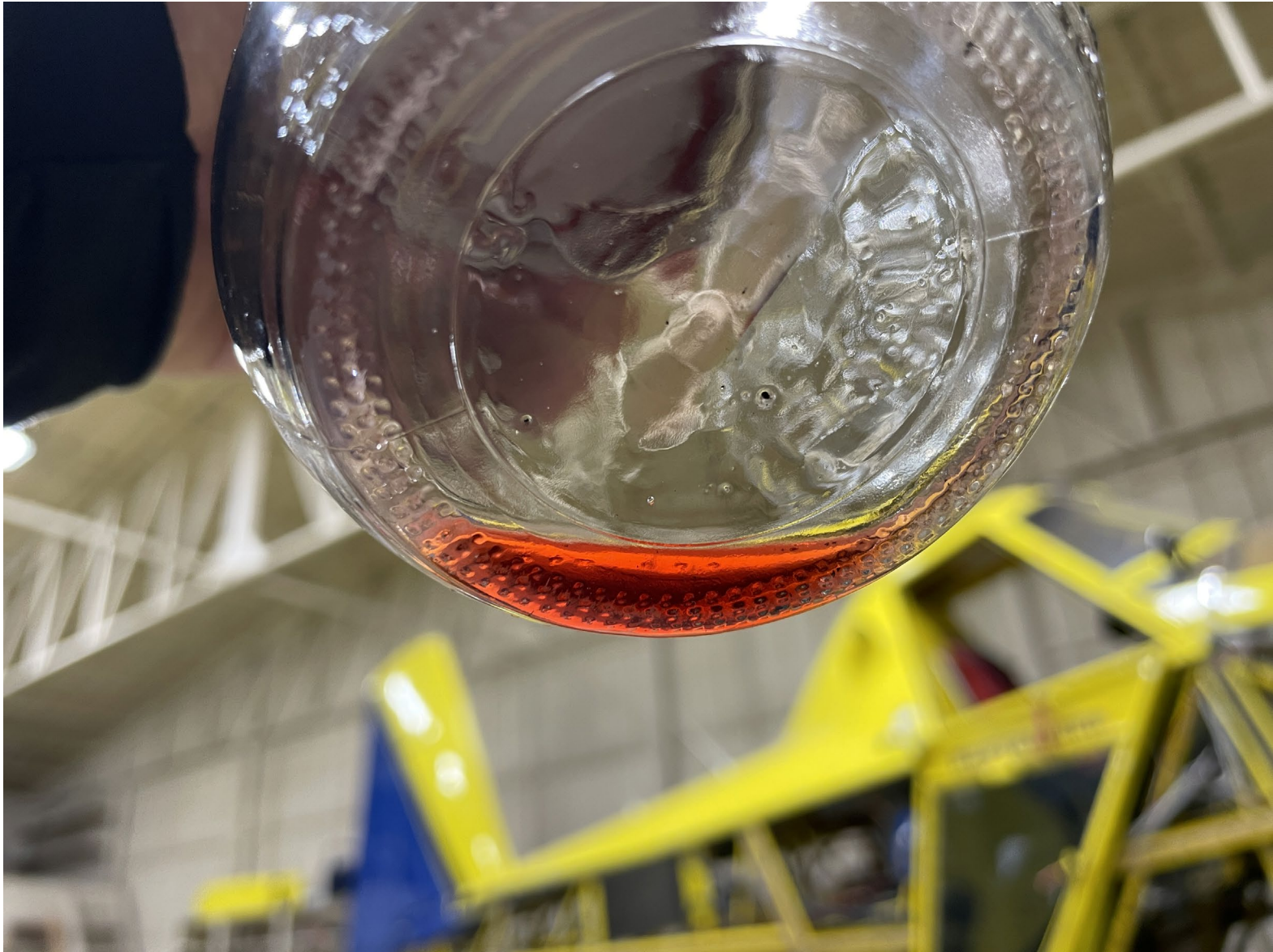
Photograph 7 - Brake fluid recovered from right brake system (Courtesy of NTSB)
