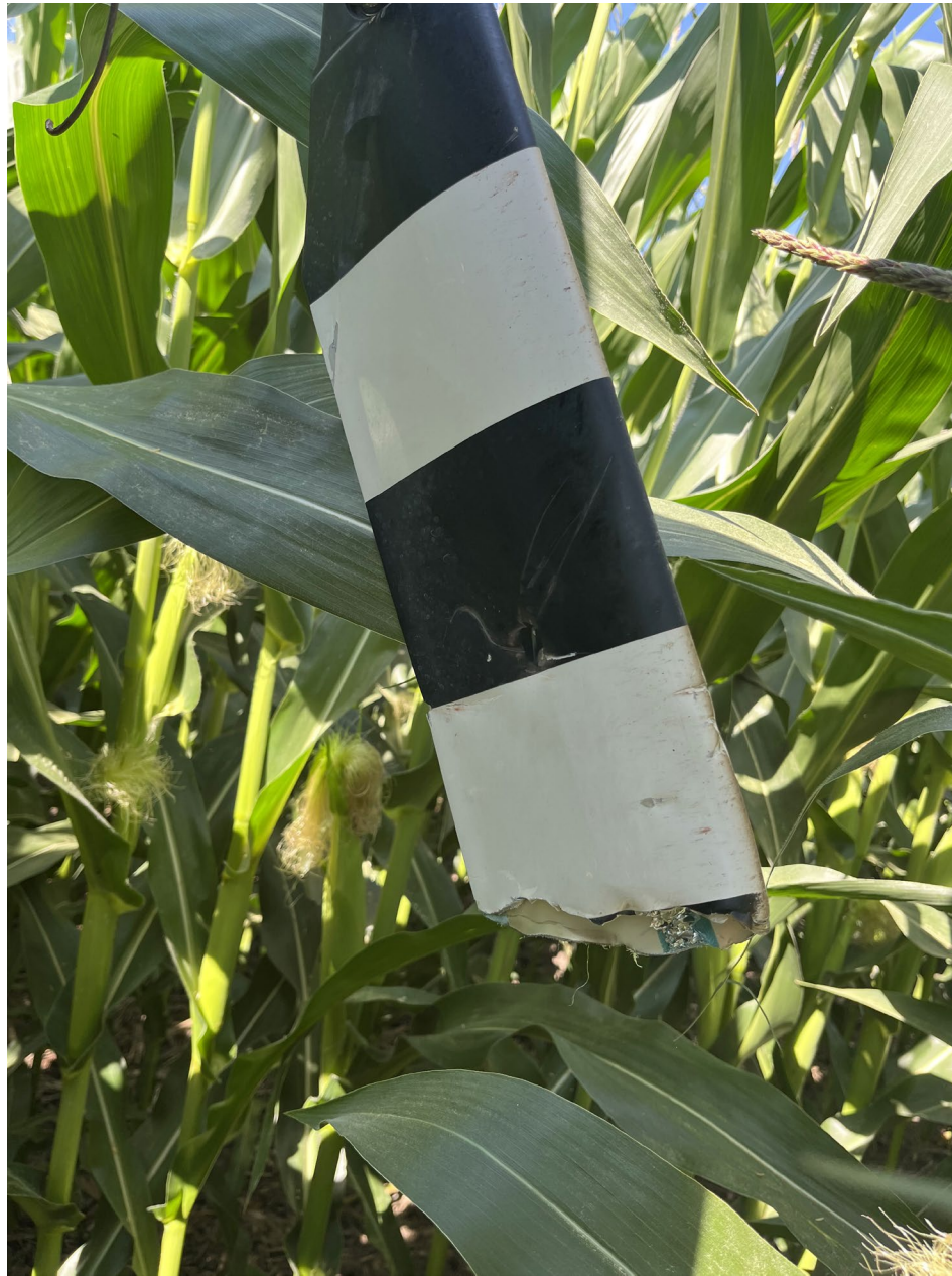
Photo 2 - Tail Rotor Blade Damage, Courtesy of FAA
