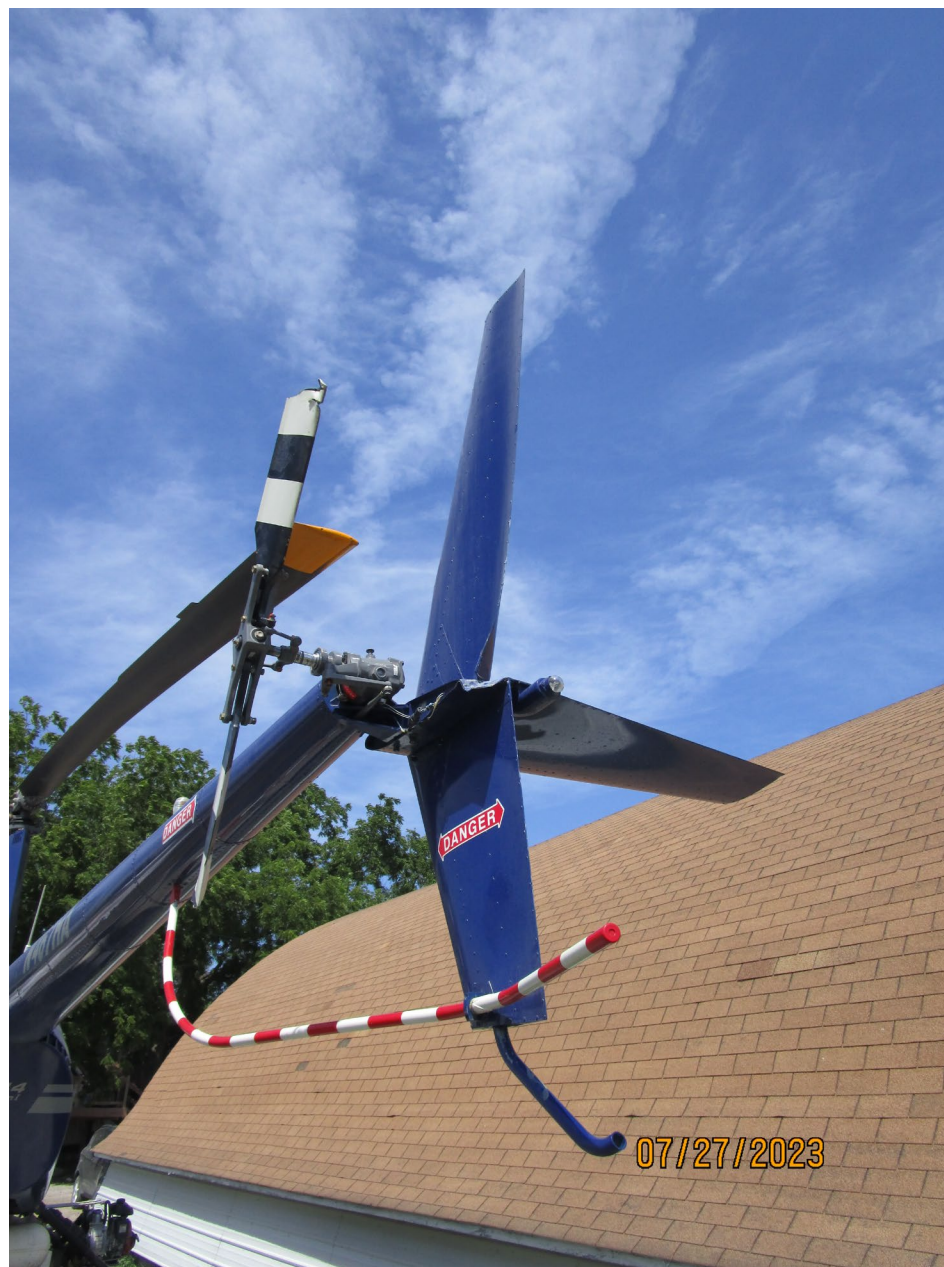
Photo 1 - Tail Rotor Blade Damage, Courtesy of FAA
