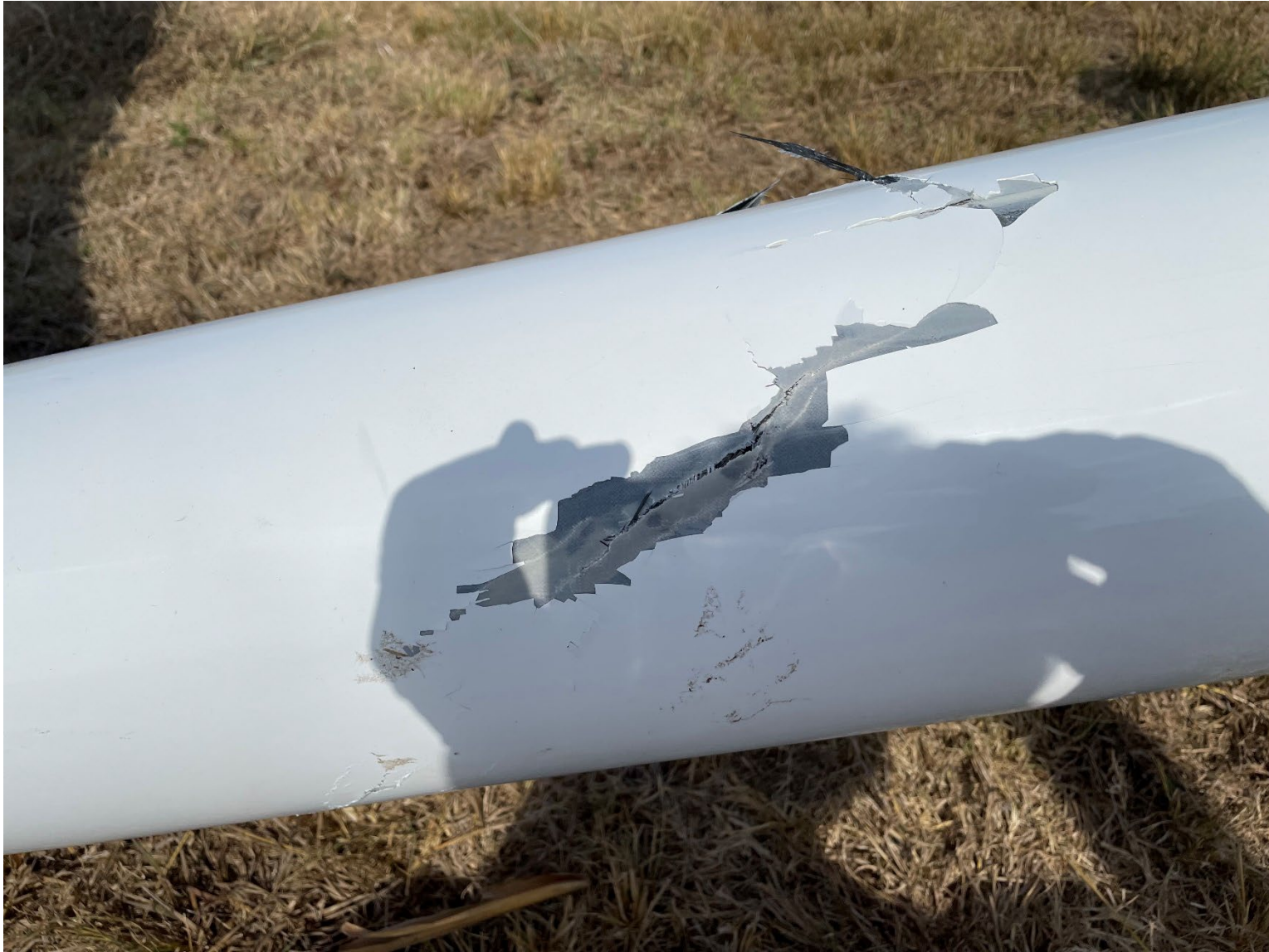
Photograph 2 - Damaged tail boom (Source: Federal Aviation Administration)
