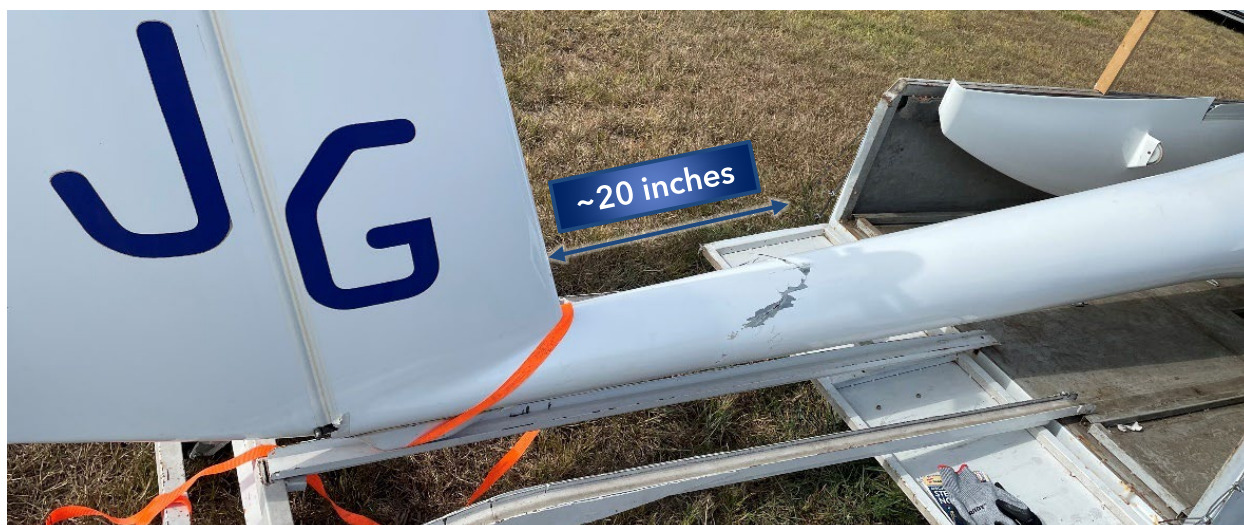
Figure 3. View of the damaged fuselage before it was sectioned from the aircraft. (Image provided by the Federal Aviation Administration)
