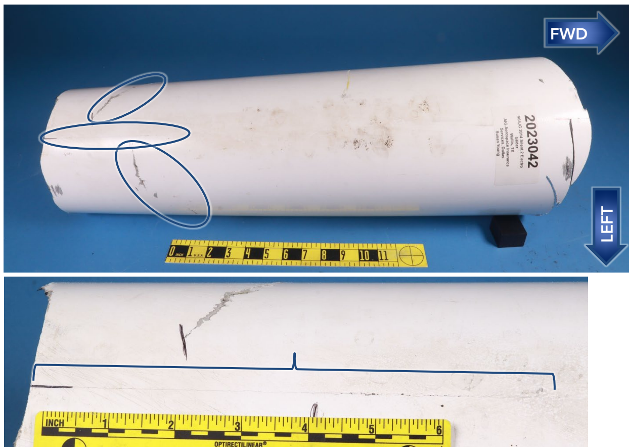
Figure 2. Overall view of the lower side of the submitted fuselage section (upper image), where locations of cracks are outlined. The lower image shows a closer view of the longitudinal crack as indicated with an unlabeled bracket after the surface was rubbed with a fine black powder to help reveal the forward end of the crack in the white paint.
