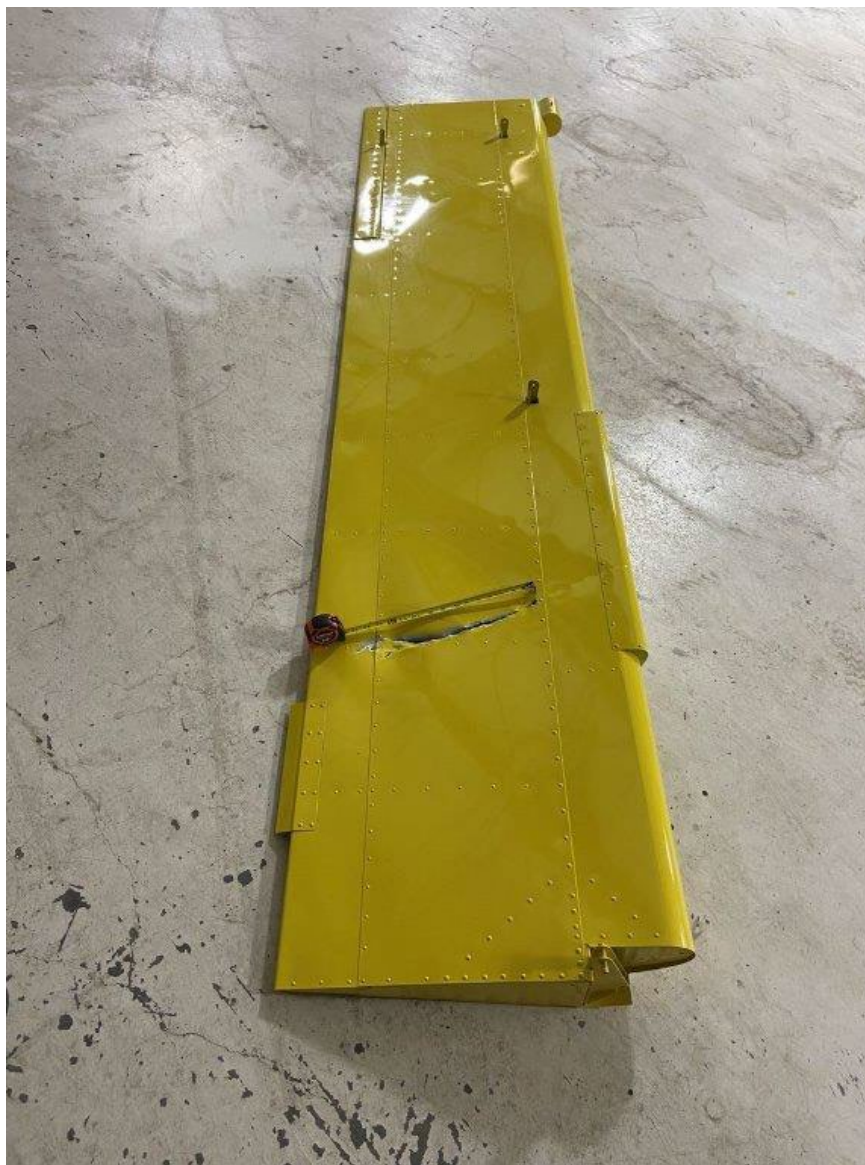
Photograph 2 - Tears to the aluminum skin of the right aileron (Courtesy of the FAA)
