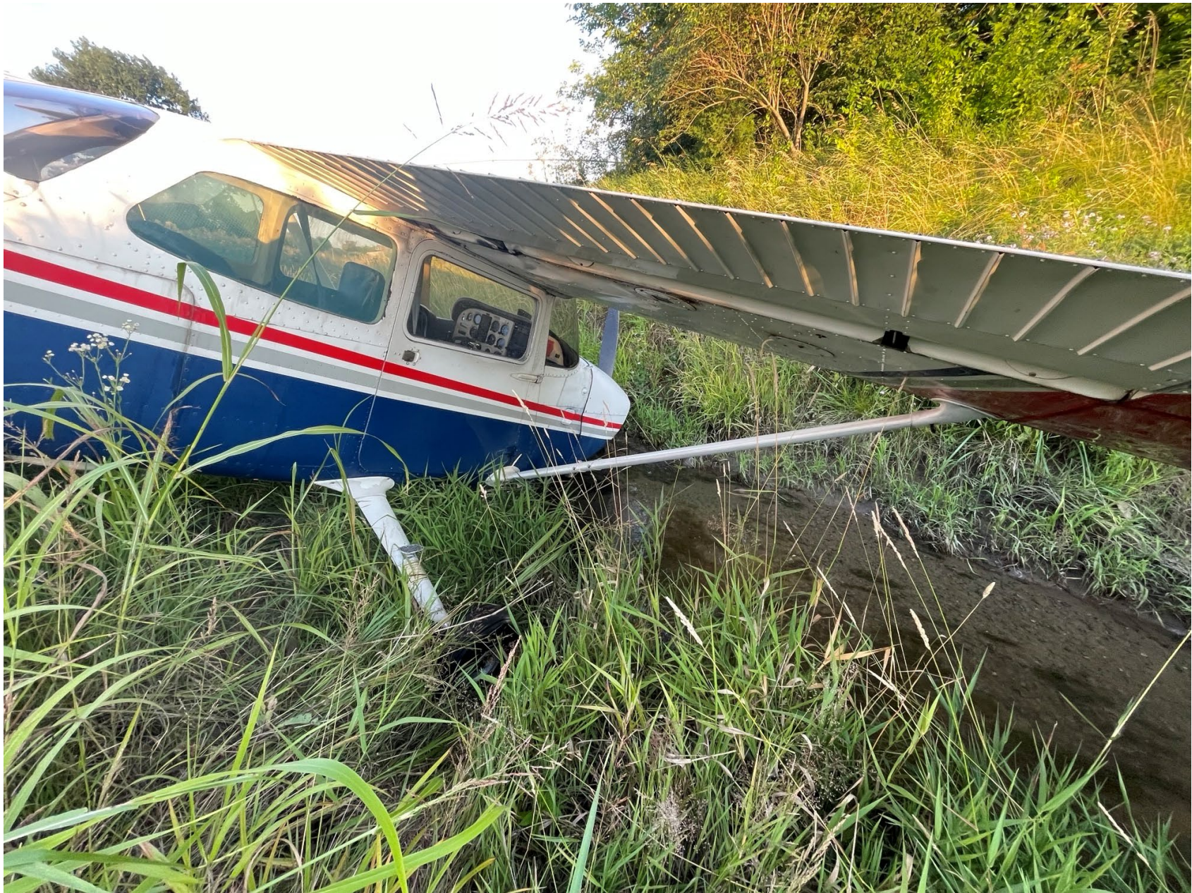
Photo 2 – Damage to inboard right wing (Source: Federal Aviation Administration)
