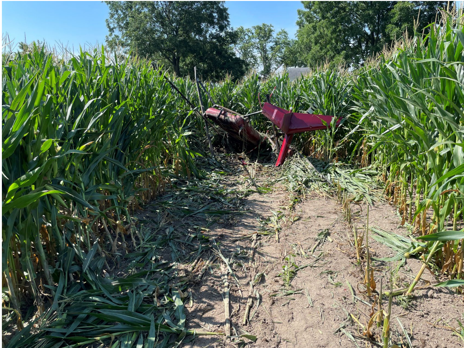
Photograph 2 - Separated landing gear and tail boom (Courtesy of Federal Aviation Administration)
