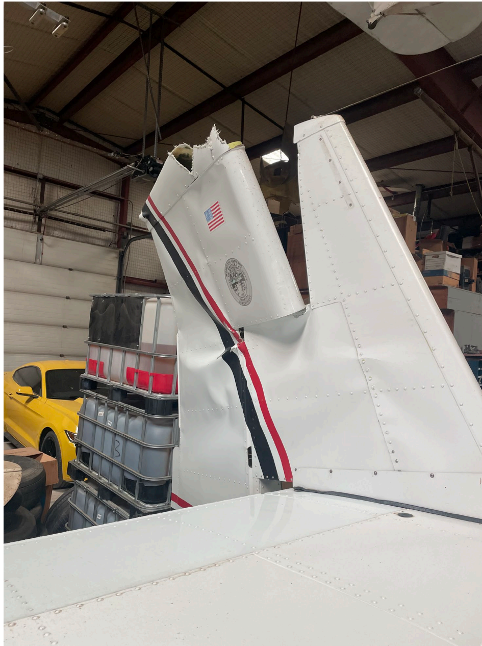
Photo of Damaged Vertical Stabilizer and Rudder, Courtesy of AA
