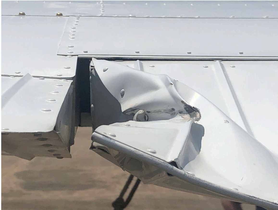
Photograph 3 - Damaged Left Flap (Courtesy of FAA)
