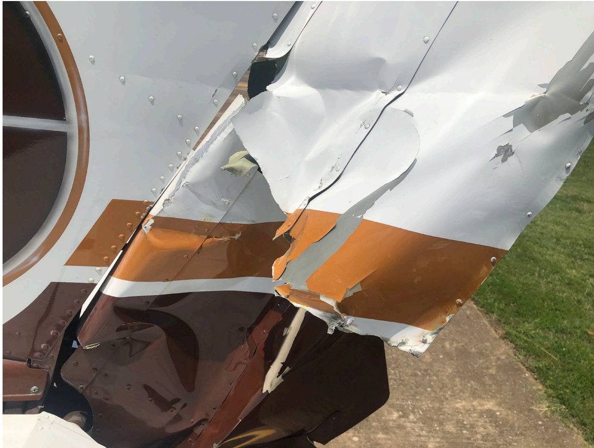
Photograph 2 - Damaged Rudder (Courtesy of FAA)
