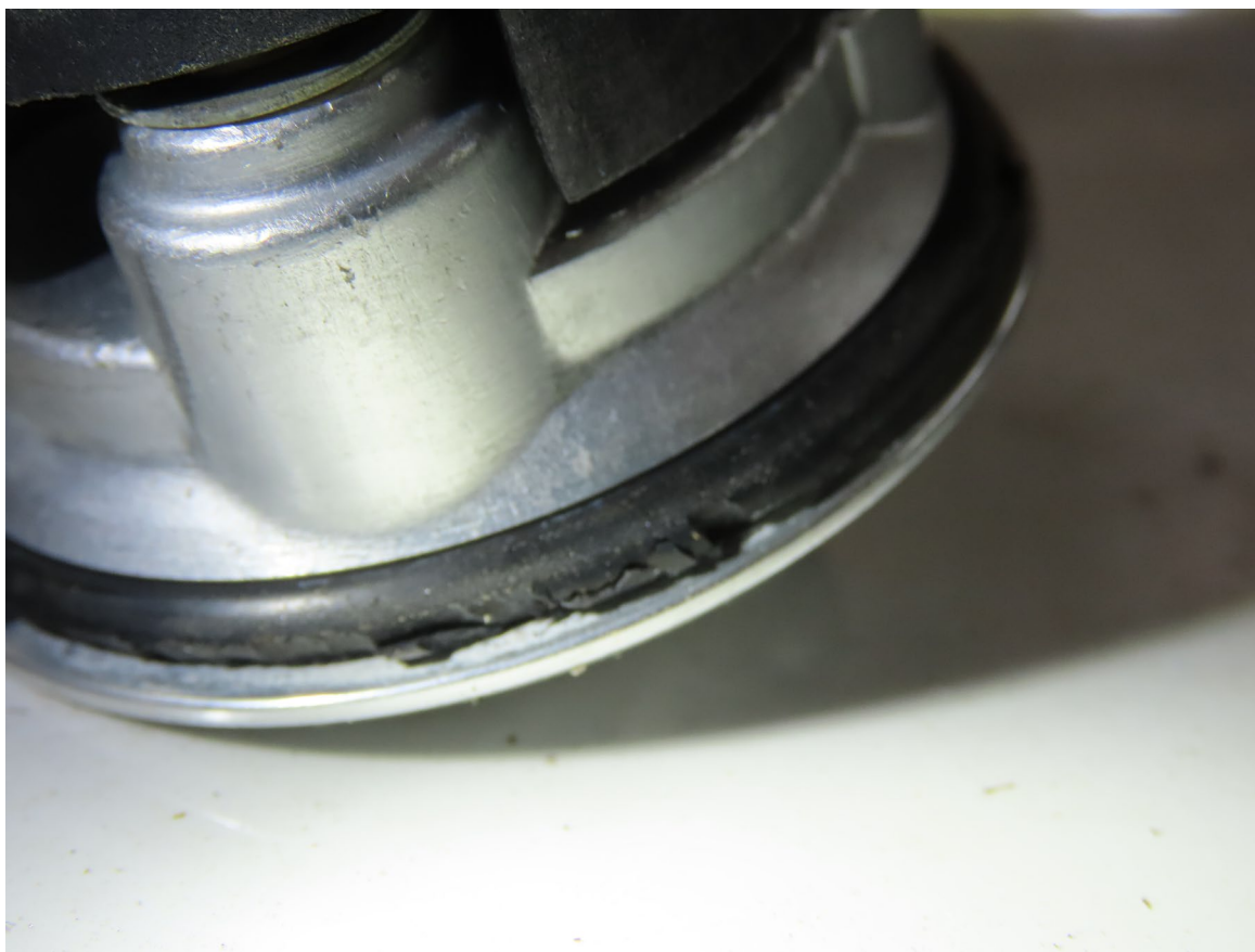
Photograph 3 - Left Fuel Cap with Cracked O-Ring (Courtesy of NTSB)
