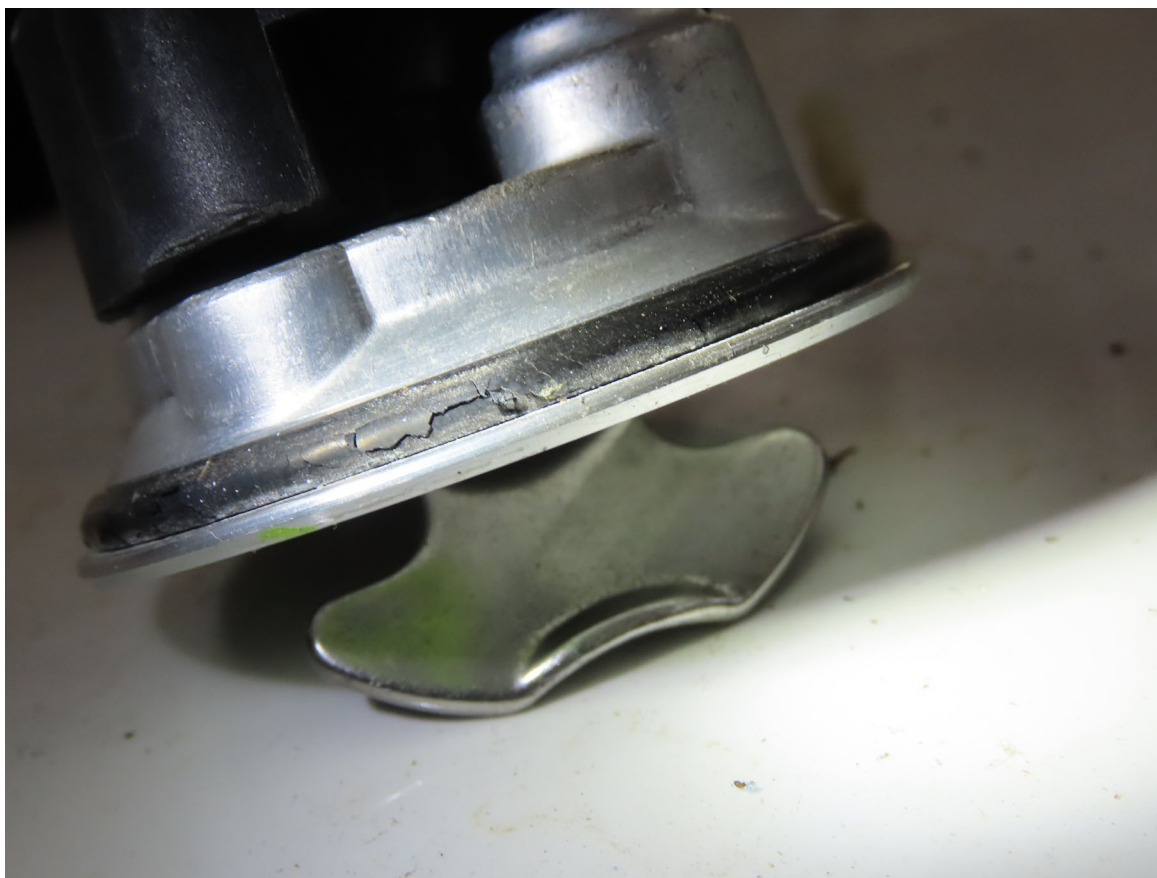
Photograph 4 - Right Fuel Cap with Cracked O-Ring (Courtesy of NTSB)
