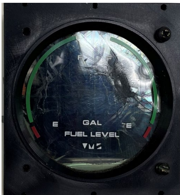
Figure 3. VM Fuel Level System Indicator as received by the NTSB Vehicle Recorder Lab.
