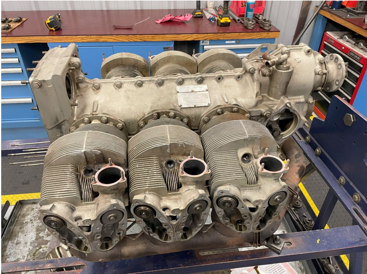
Figure 1. Left engine during teardown Examination (NTSB Photo)
