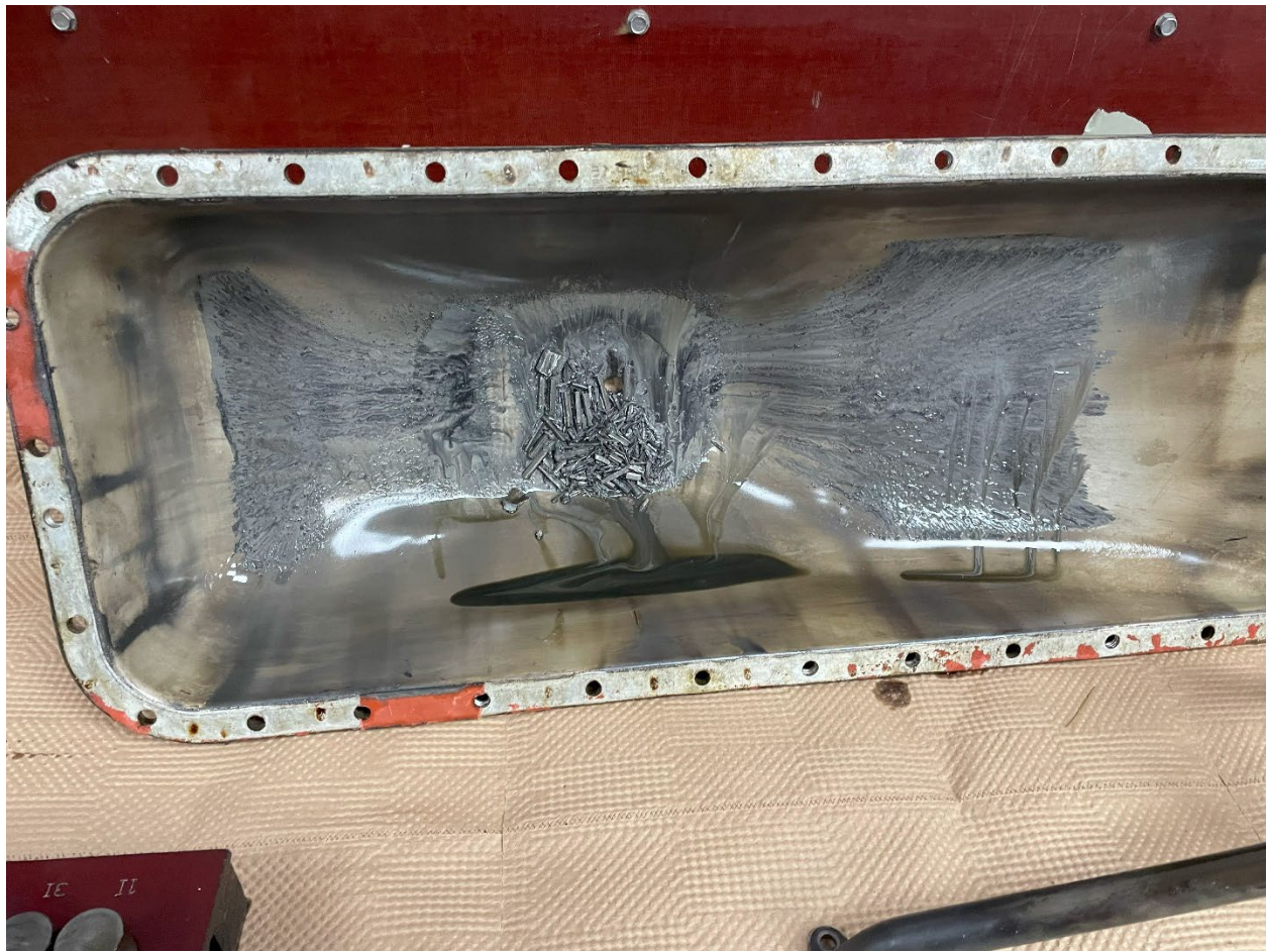
Figure 4. Remnants of gear teeth in engine oil sump. (NTSB Photo)
