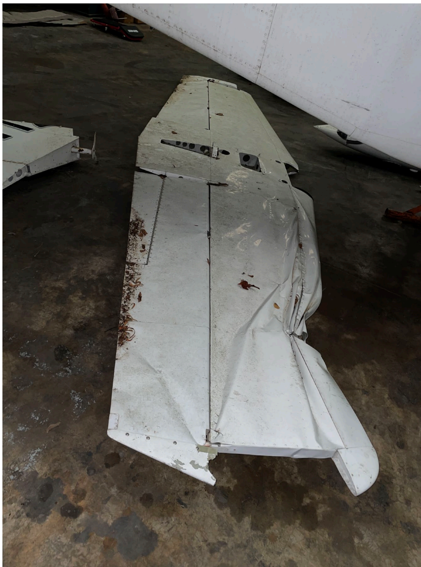
Photograph 3 - Stabilizer during postaccident examination (NTSB Photo)
