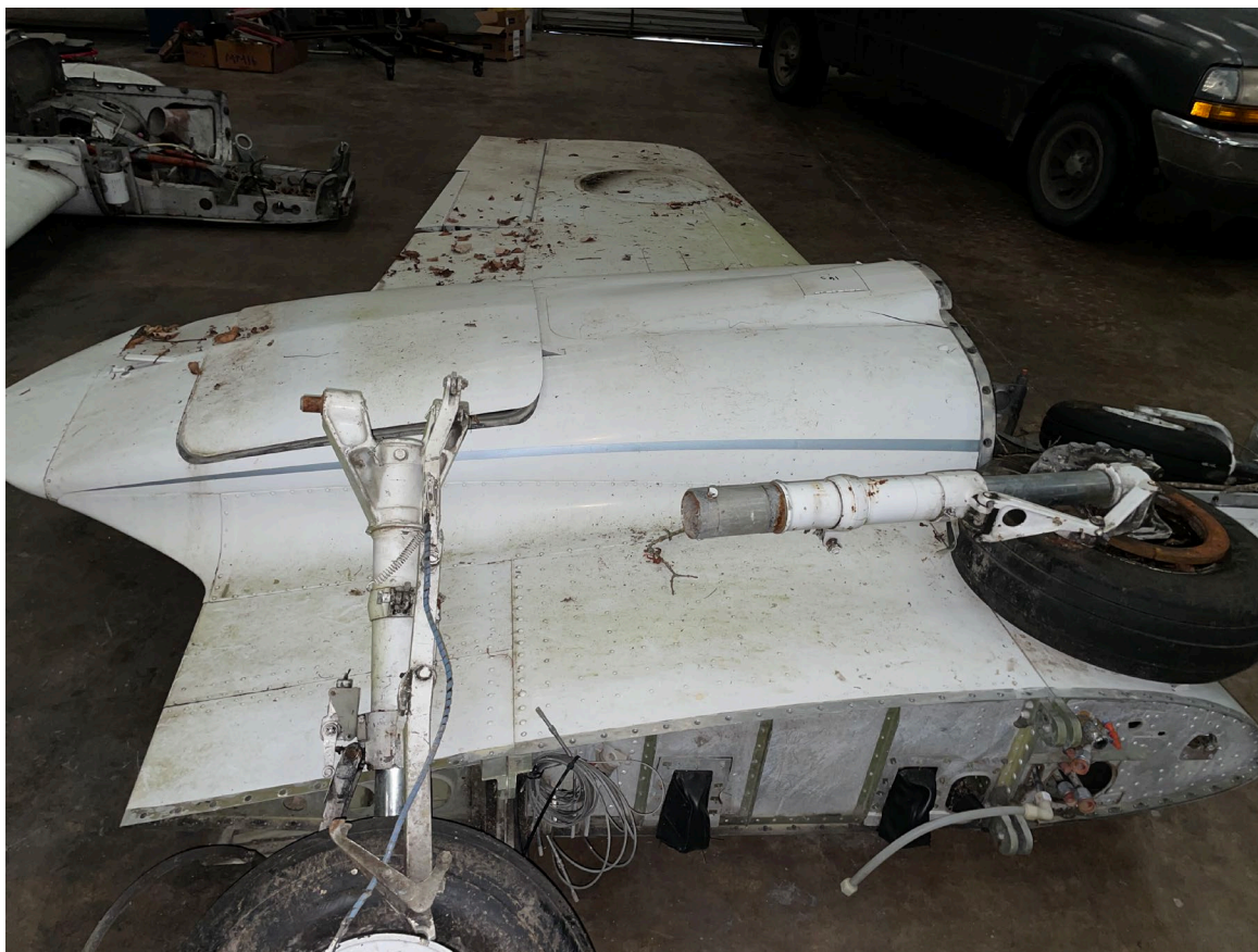
Photograph 5 - Left wing during postaccident examination (NTSB Photo)
