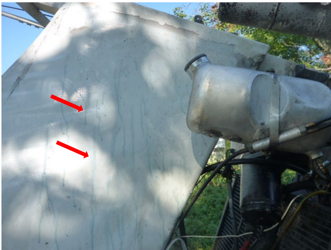
Photograph 2 - Injection Oil Spray (Taken by NTSB)
