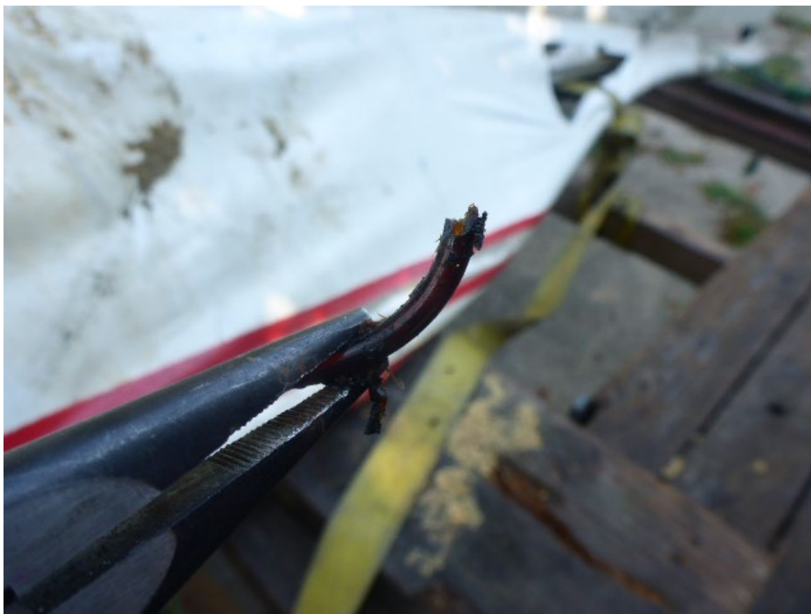
Photograph 6 - Fragment of Old Oil Injection Line (Taken by NTSB)
