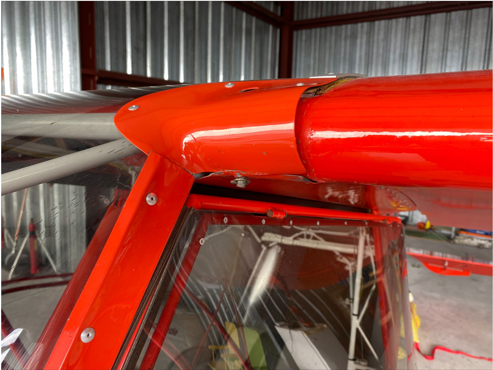
Photo 2 – Left wing damage (Source: Accident Pilot)
