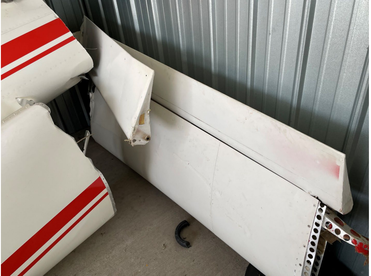
Figure 6. Separated section of left wing and left aileron.
