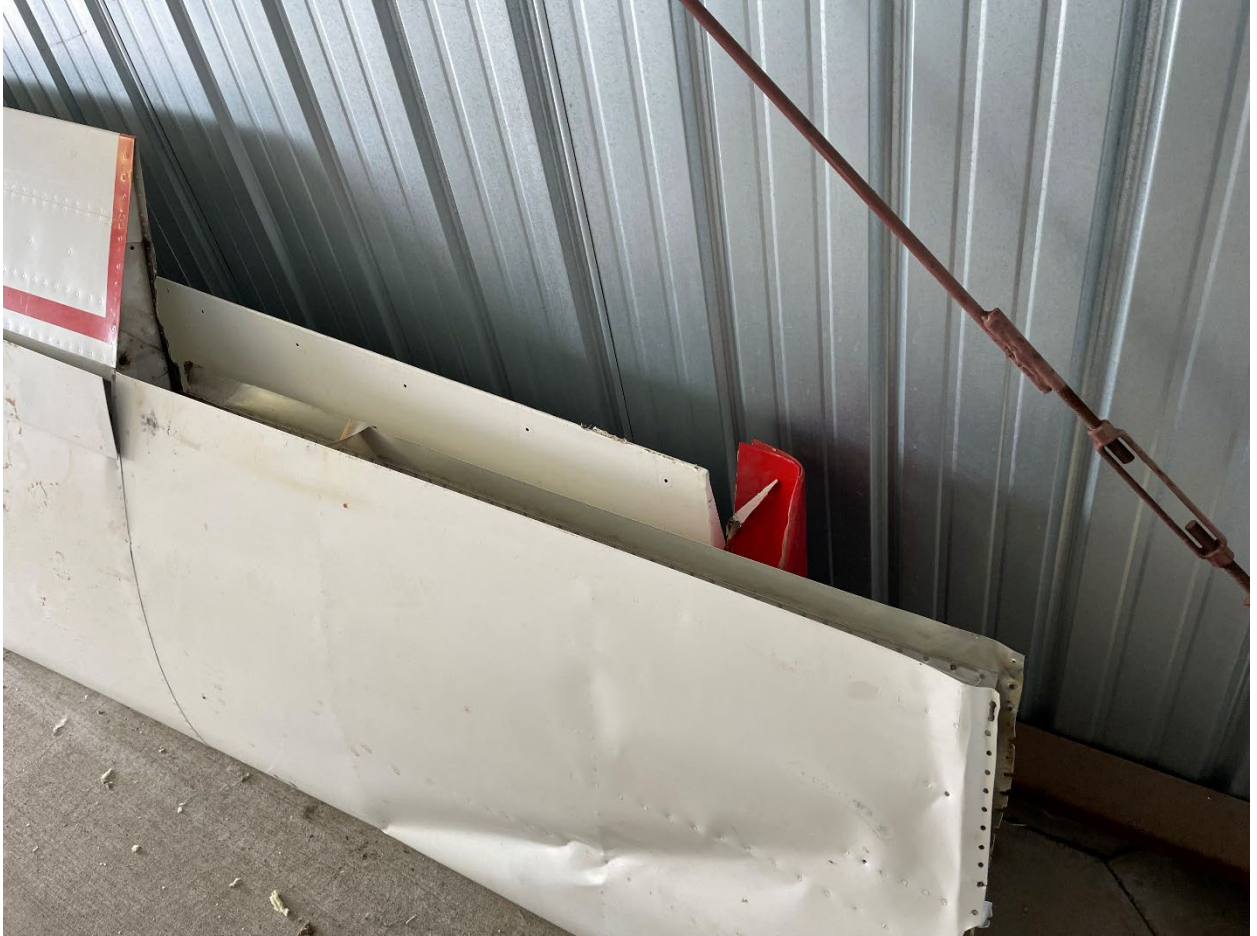
Figure 5. Photo showing the end of the left wing at the separation location.
