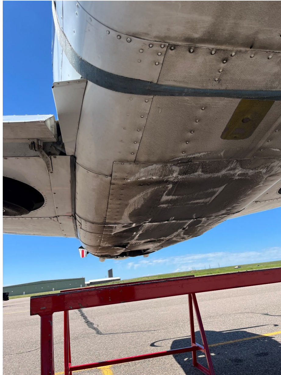
Photo 2 – Belly Damage to the Airplane (Source: Airport Manager)
