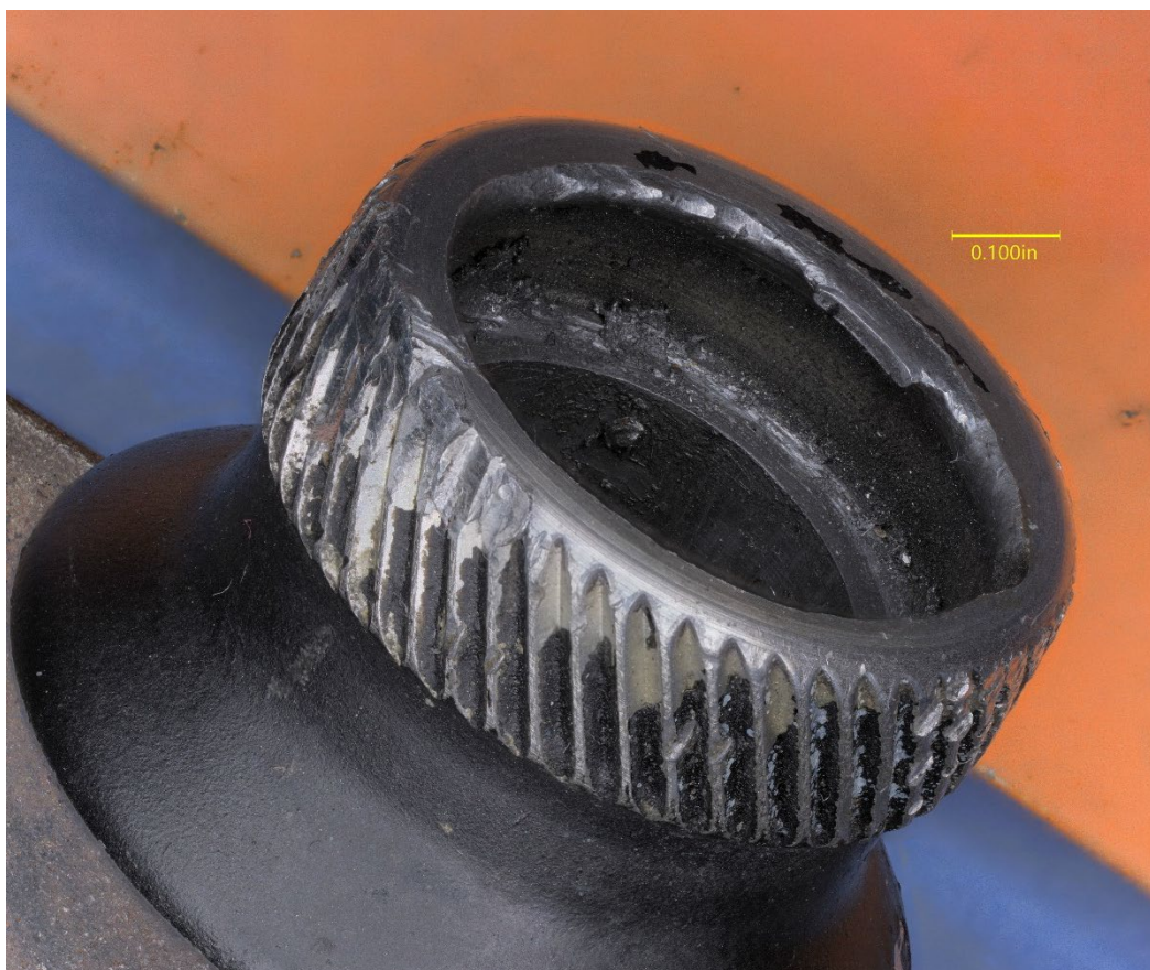
Figure 4. End cap exhibiting worn retention lip.
