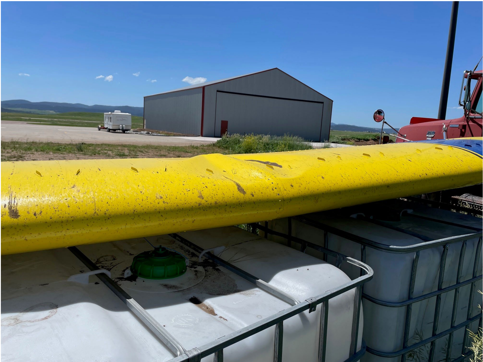
Photo 8 – View of the substantial damage sustained to the left wing (courtesy of the Federal Aviation Administration).
