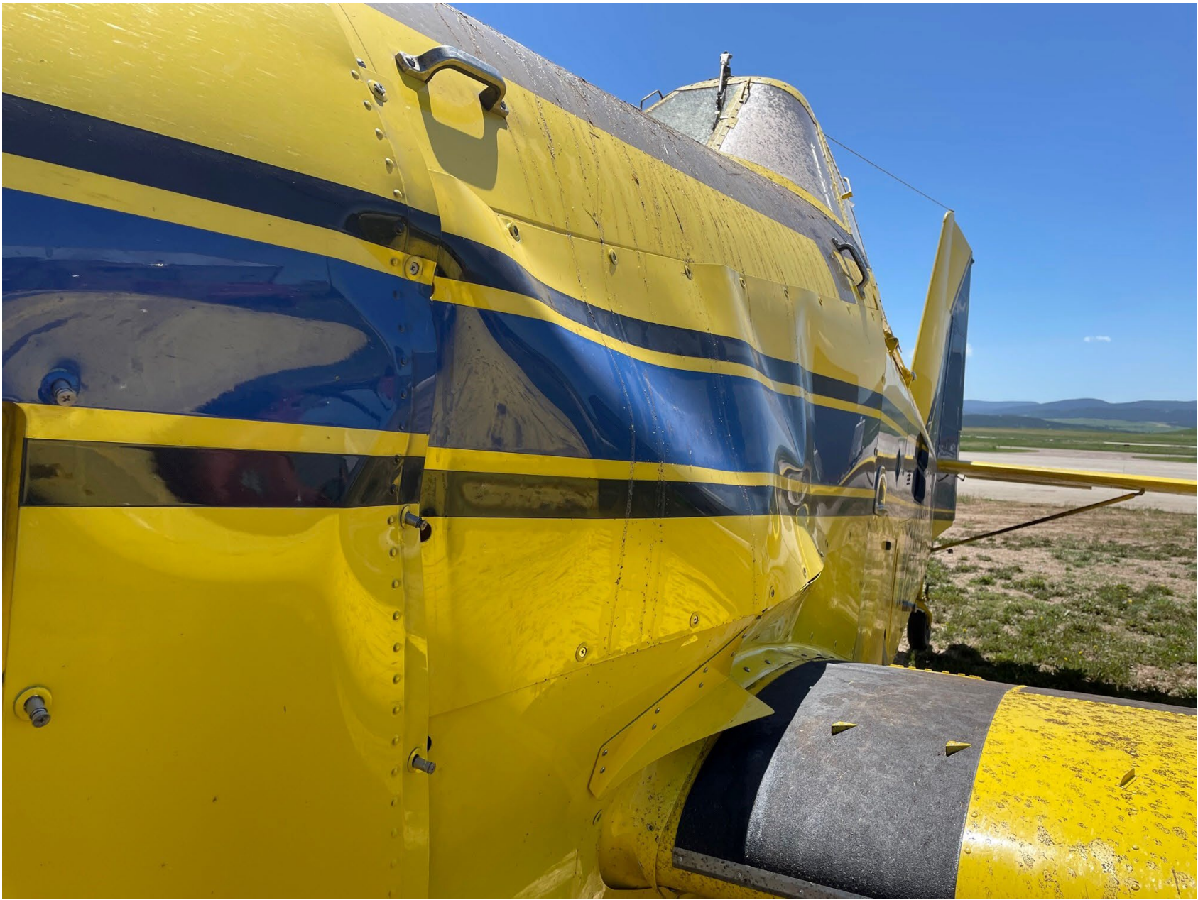
Photo 6 – View of the substantial damage sustained to the fuselage (courtesy of the Federal Aviation Administration).
