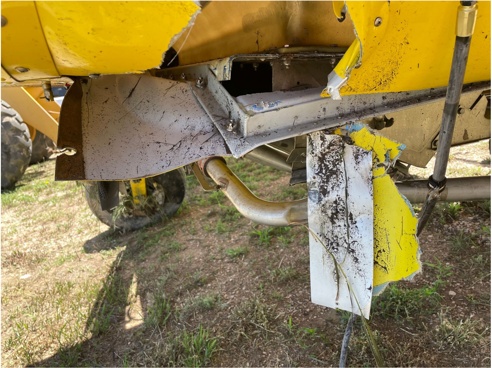
Photo 7 – View of the substantial damage sustained to the fuselage (courtesy of the Federal Aviation Administration).
