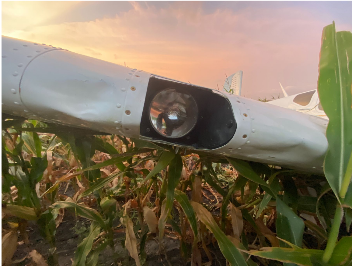
Photograph 2 - Right Wing Damage (Courtesy of Texas Division of Emergency Management)
