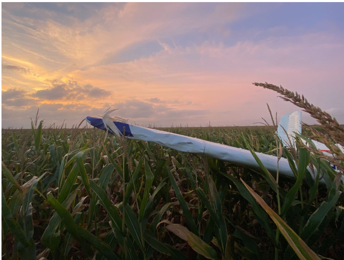
Photograph 3 - Right Wing Damage (Courtesy of Texas Division of Emergency Management)
